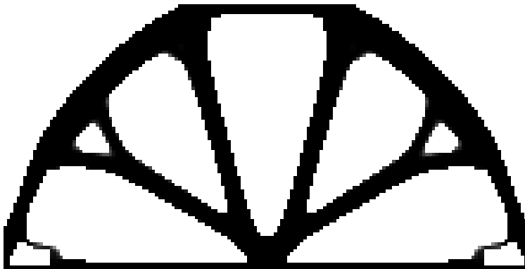
Figure 3.15: Michell truss optimal topology.
