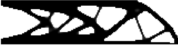
Figure 3.13: Unsymmetric cantilever optimal topology.
