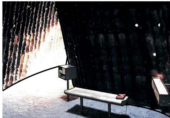
This formwork is later on removed by burning it. This gives the inside a rough burned appearance (figure 4.2.5A)
