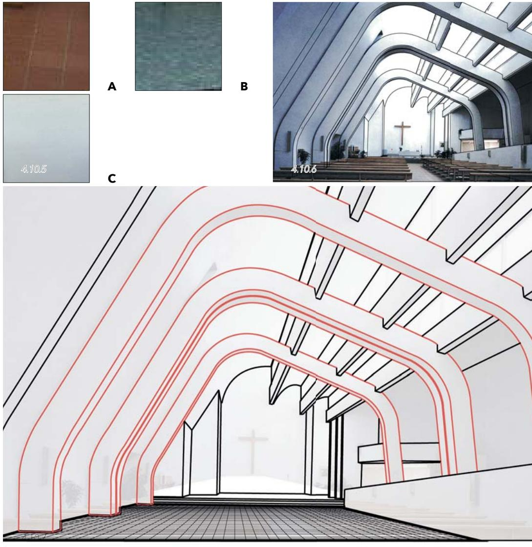
those ribs beams are positioned. Between the beams and the shelved roof window frames are situated. These openings are letting light inside the church at the top of the space. This light is entering above the user thence it feels like a holy space.
