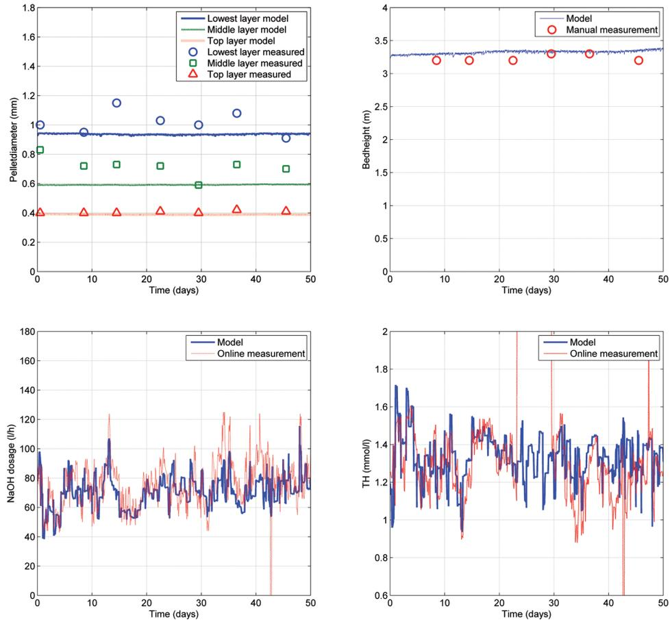
**Figure 4.4.** Validation results for reactor 4. Pellet size distribution (top left), bed height (top right), NaOH dosage (bottom left) and TH (bottom right).
