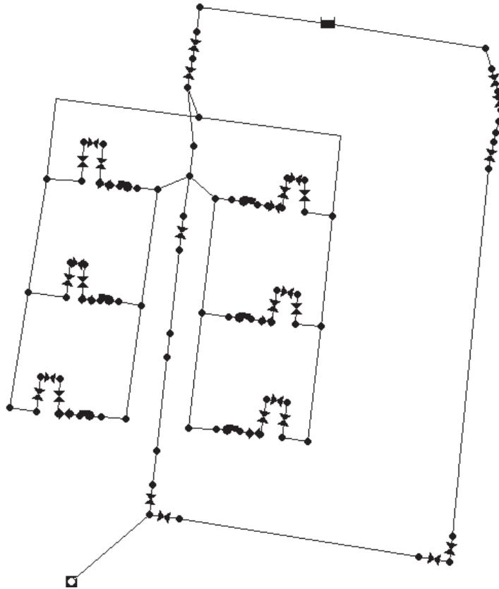
Figure 3.5. EPANET model of the softening plant and raw water supply of Wim Mensink.
