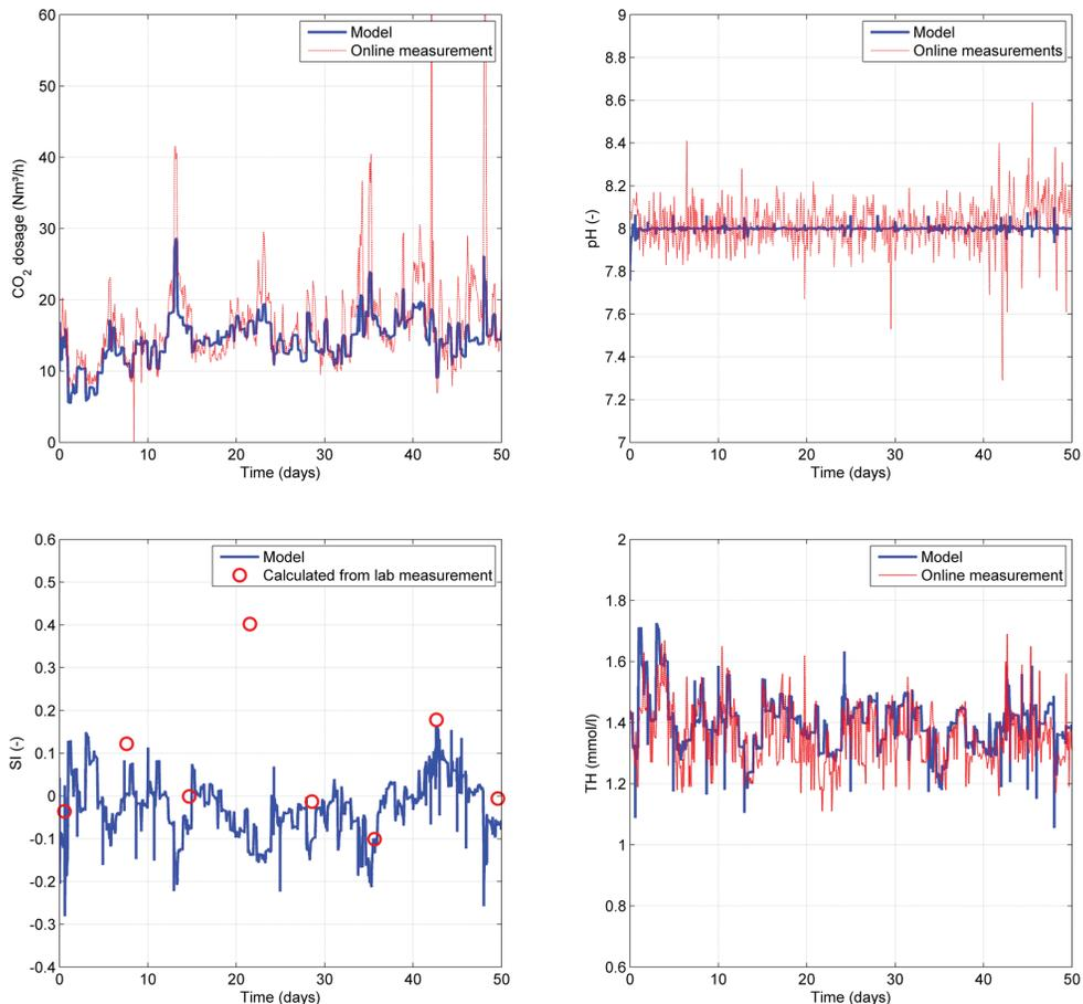
**Figure 4.5.** Results validation Lane 1.  $\text{CO}_2$  dosage (top left), pH (top right), SI (bottom left) and TH (bottom right).
