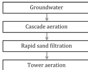
**Figure 3.2.** Treatment scheme of drinking water treatment plant Harderbroek
