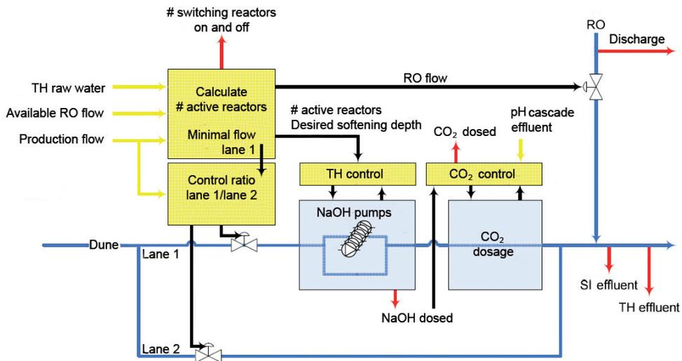
**Figure 4.3.** Control configuration for the Wim Mensink case. Blue lines are the water flows, yellow arrows are the online measured parameters. Red arrows are the controlled variables, black arrows are the control actions.
