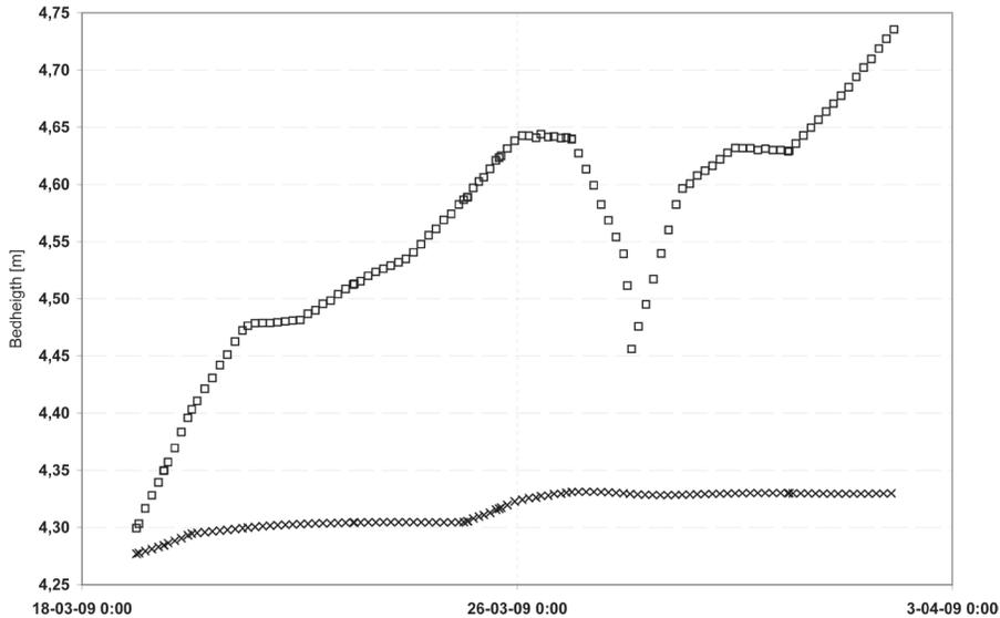
**Figure 2.5.** Selection of results from the case study as generated by the simulator: bed height with the former control (□) and the new control (×) during decreasing water temperature.
