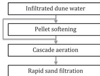
**Figure 3.4.** Treatment scheme of drinking water treatment plant Wim Mensink
