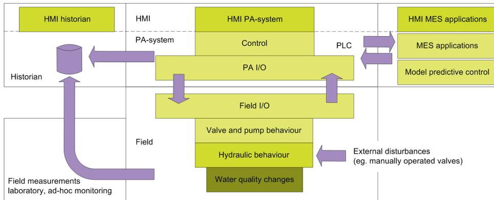
**Figure 1.2.** Typical setup of a PA-system, the field, the human-machine interface (HMI), the manufacturing execution systems (MES applications) and the historian containing data. I/O stands for input/output.
