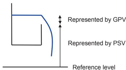
**Figure 3.1.** Modeling of the upper weir of a cascade aerator.
