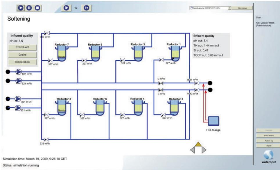
**Figure 2.4.** GUI of the pellet softening process and an example of dynamic process data. For the purpose of this thesis, the original Dutch texts have been replaced by English.
