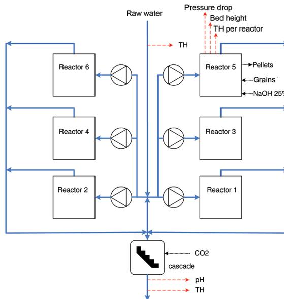
Figure 4.2. Detail of the layout of the pellet softening treatment step. Blue lines are water flows, red dotted arrows are online measurements, small black arrows are control actions. TH is total hardness.
