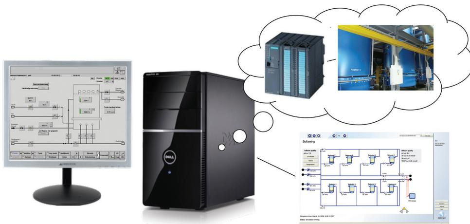
**Figure 1.4.** Process models connected to the emulated PA-software. The 'behavior' of the plant is added
