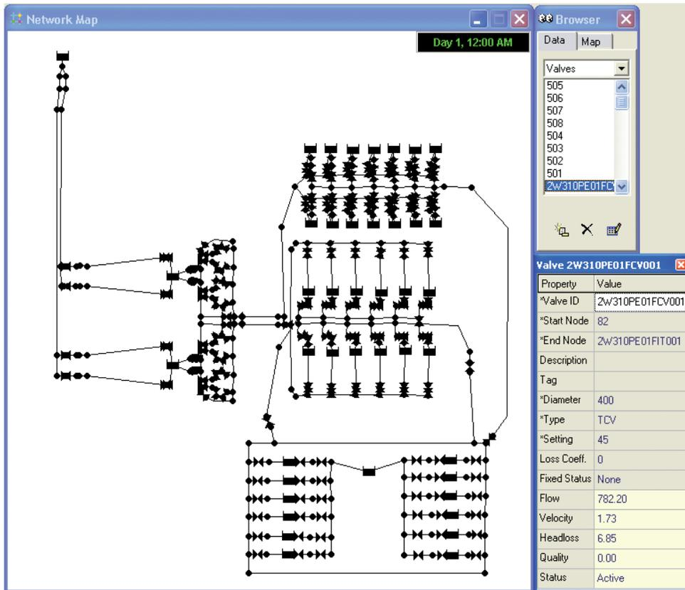
Figure 2.3. EPANET model for the drinking water treatment plant at Weesperkarspel.
