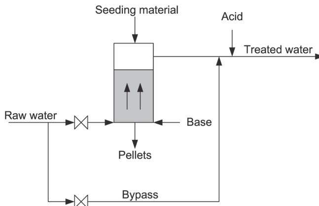
**Figure 5.1.** Bypass of water in pellet softening (van Schagen *et al.*, 2008).
