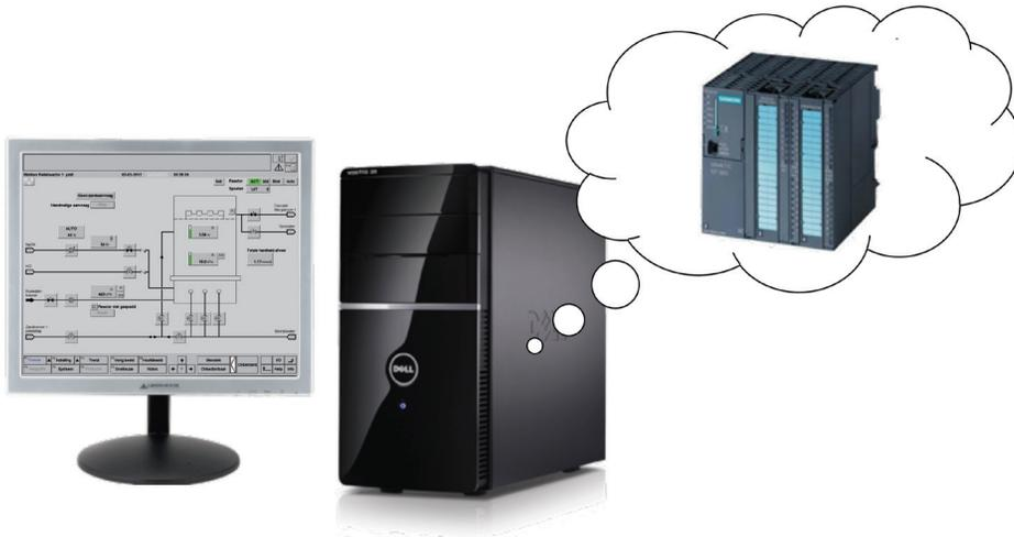
**Figure 1.3.** Emulation of PA-software. A PC imitates a PLC, indistinctive for the PA-software.
