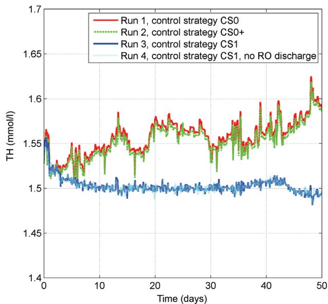
**Figure 4.7.** TH in the clear water reservoir for run 1 and 2 (upper lines) and for runs 3 and 4 (lower lines).
