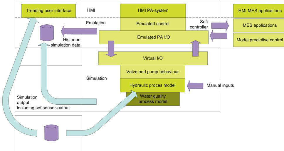
**Figure 1.5.** The virtual representation of the PA-system and field. HMI is human machine interface, MES is the manufacturing execution system, I/O stands for input/output.
