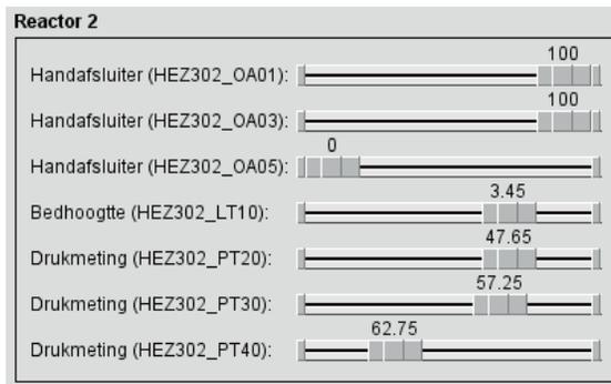
Figure 6.3. Virtual sliders for sensors and actuators of Reactor 2 in the VC-system (labels in Dutch, 'Handafsluiter' is manually operated valve, 'Bedhoogtte' is bed height, and 'Drukmeting' is pressure measurement).
