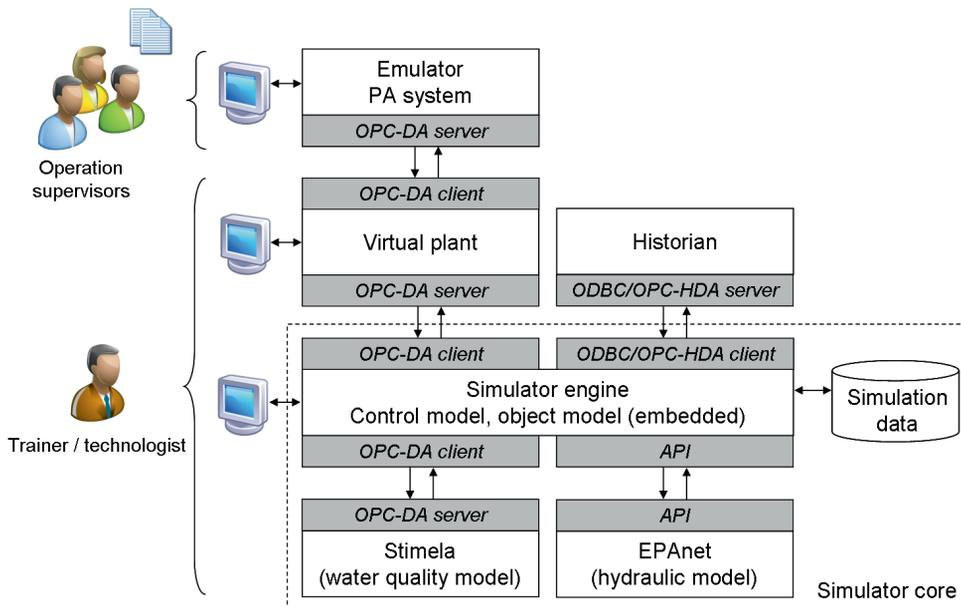
Figure 2.1. Simulator's software structure.
