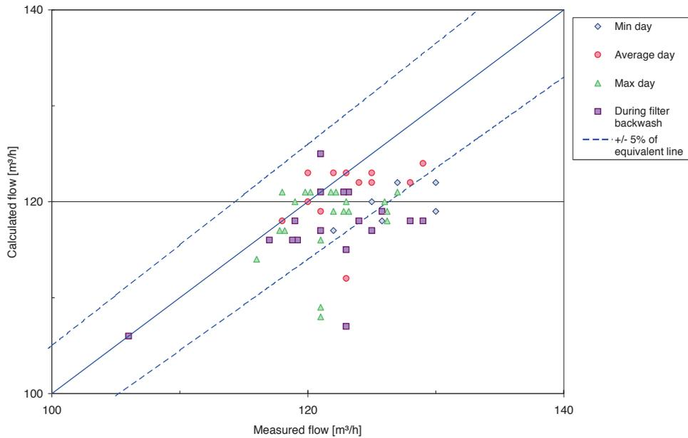
Figure 3.6. Validation results of flows from wells at Harderbroek.
