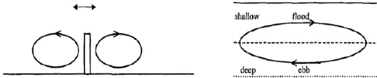
Figure 2-5. Geometry induced (left) and bathymetry induced (right) circulation
