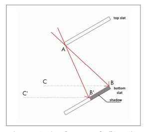
Figure 41. Section of two rows of collectors in a stack array.
