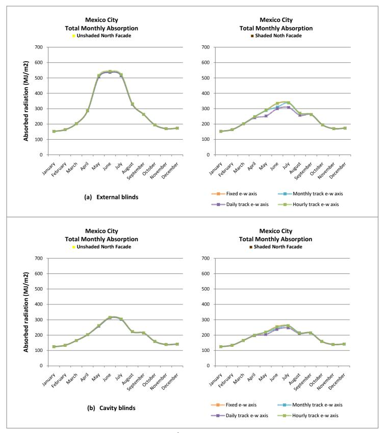
Figure 63. Absorption per m<sup>2</sup> of absorber surface for North Façade.
