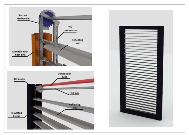
Figure 110. Tiltable and retractable blind
