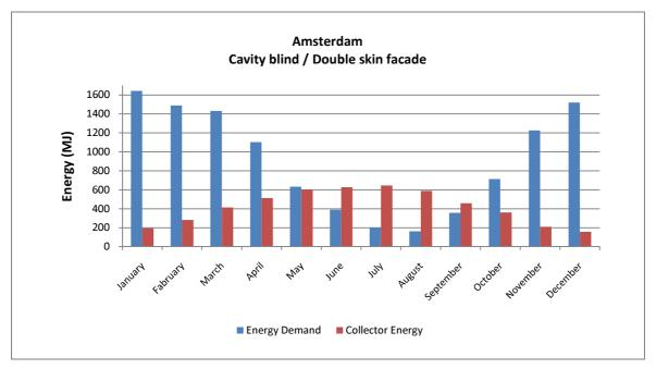
Figure 85. Energy demand and collector energy output for shaded cavity blinds.
