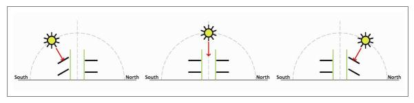
Figure 37. Slope angle  $\beta$  of slats when no solar radiation is falling on a particular façade.
