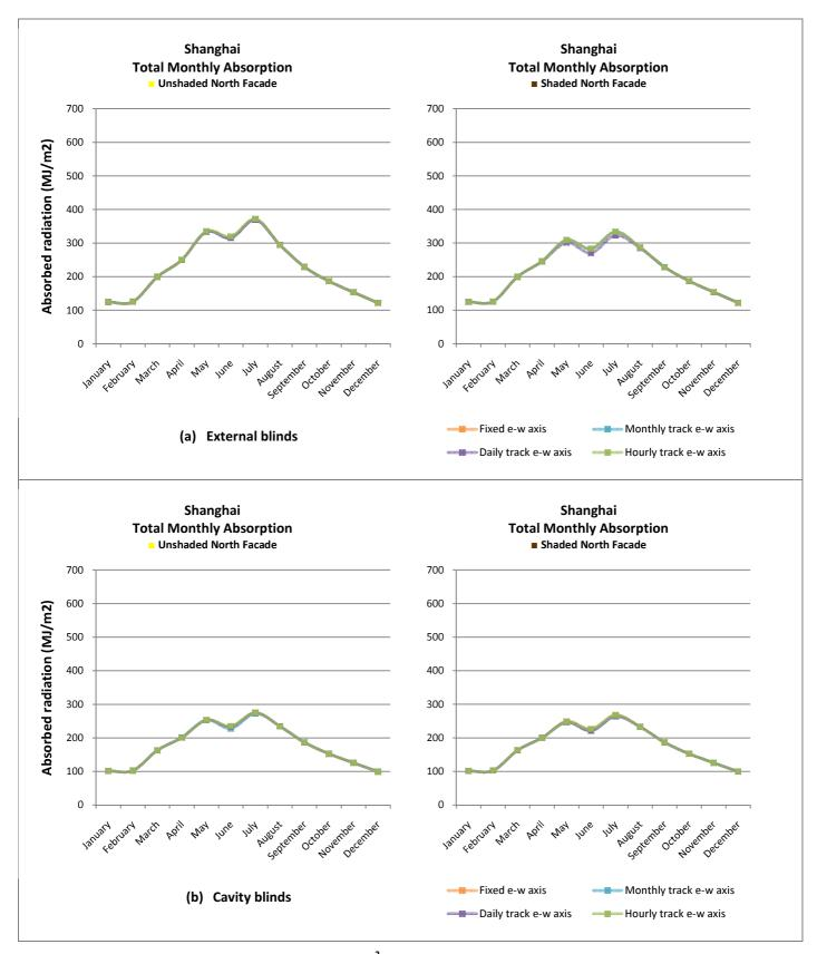
Figure 67. Absorption per m<sup>2</sup> of absorber surface for North Façade.
