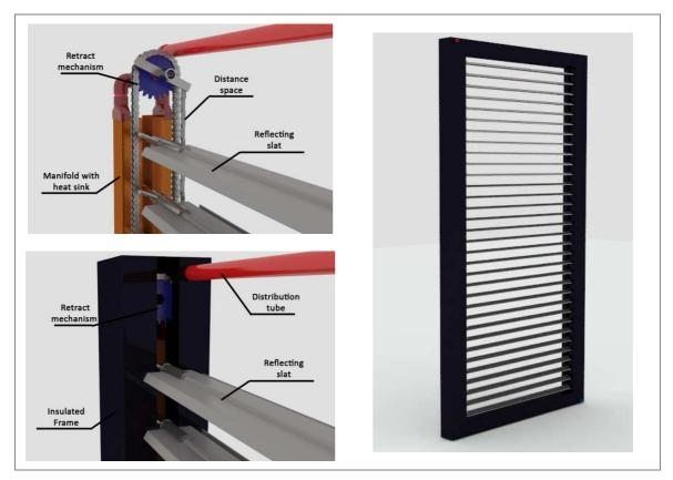
Figure 109. Fixed-angle retractable blind.
