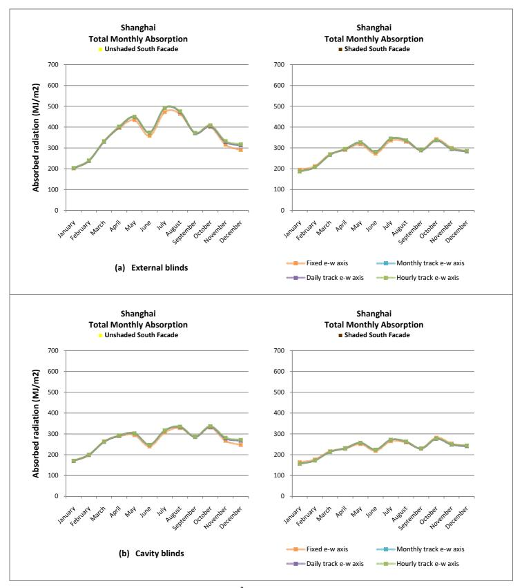
Figure 66. Absorption per m<sup>2</sup> of absorber surface for South Façade.
