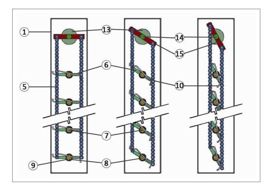
Figure 118. Tilting mechanism for tracking blind.
