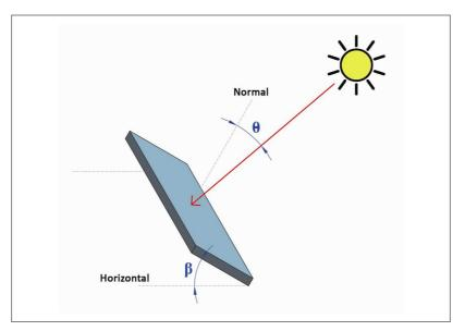
Figure 35. Angle of incidence  $\theta$  of radiation on a surface and slope angle  $\beta$  of collector.
