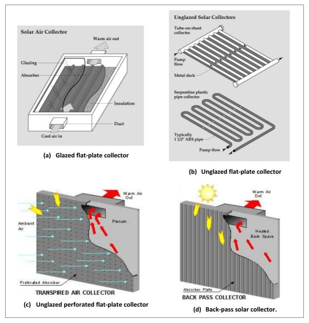
Figure 10. Air based solar collectors (Encyclopedia of Alternative Energy and Sustainable Living, 2010).
