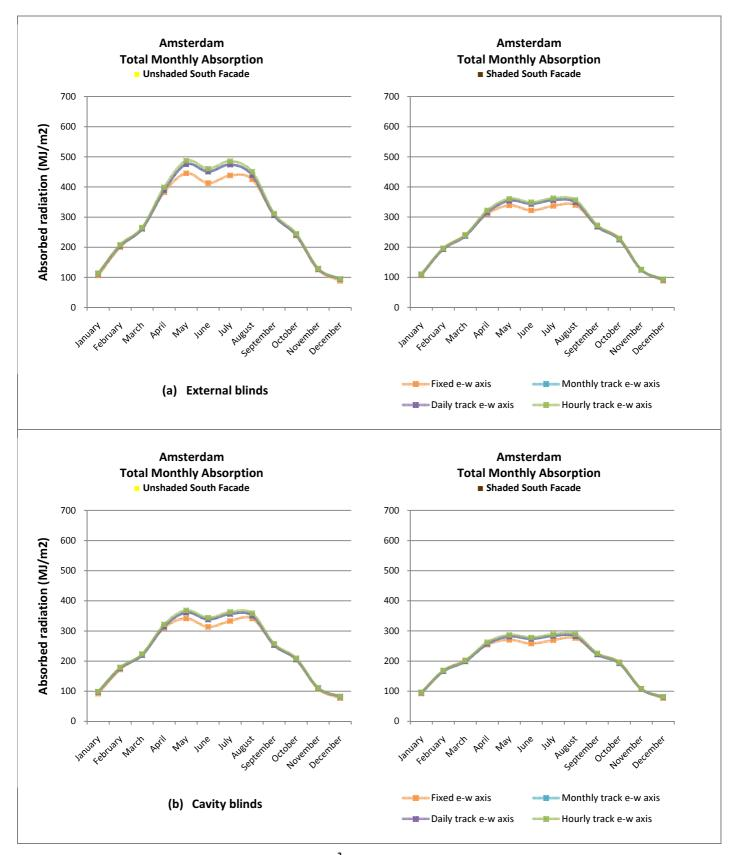
Figure 74. Absorption per m<sup>2</sup> of absorber surface for South Façade.
