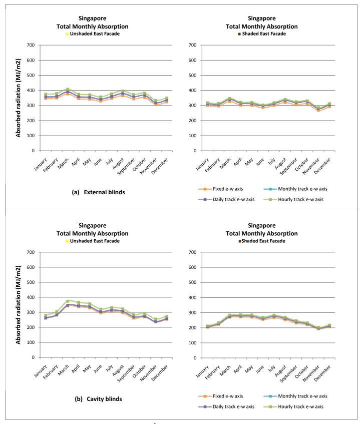
Figure 56. Absorption per m<sup>2</sup> of absorber surface for East and West Facade.
