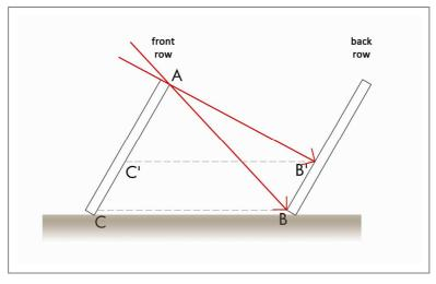
Figure 40. Section of two rows flat-plate collectors fixed on the ground.
