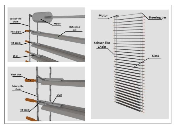
Figure 101. Tilt mechanism
