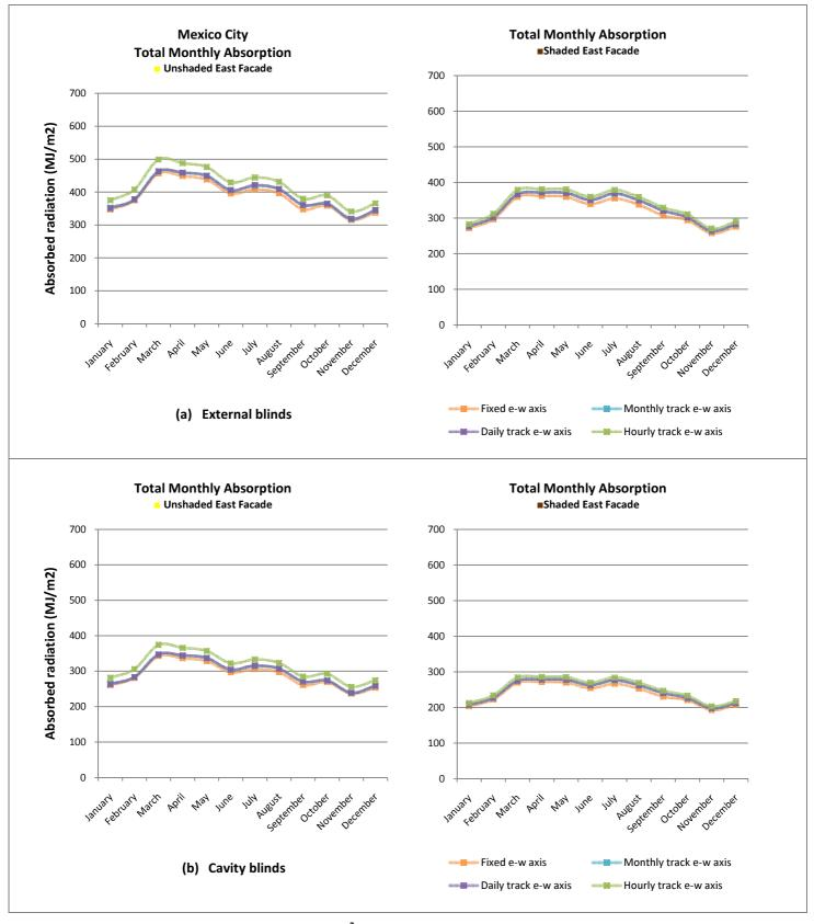
Figure 64. Absorption per m<sup>2</sup> of absorber surface for East and West Façade.
