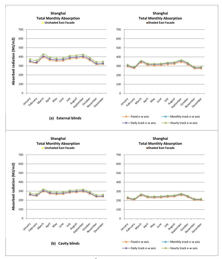
Figure 68. Absorption per m<sup>2</sup> of absorber surface for East and West Façade.
