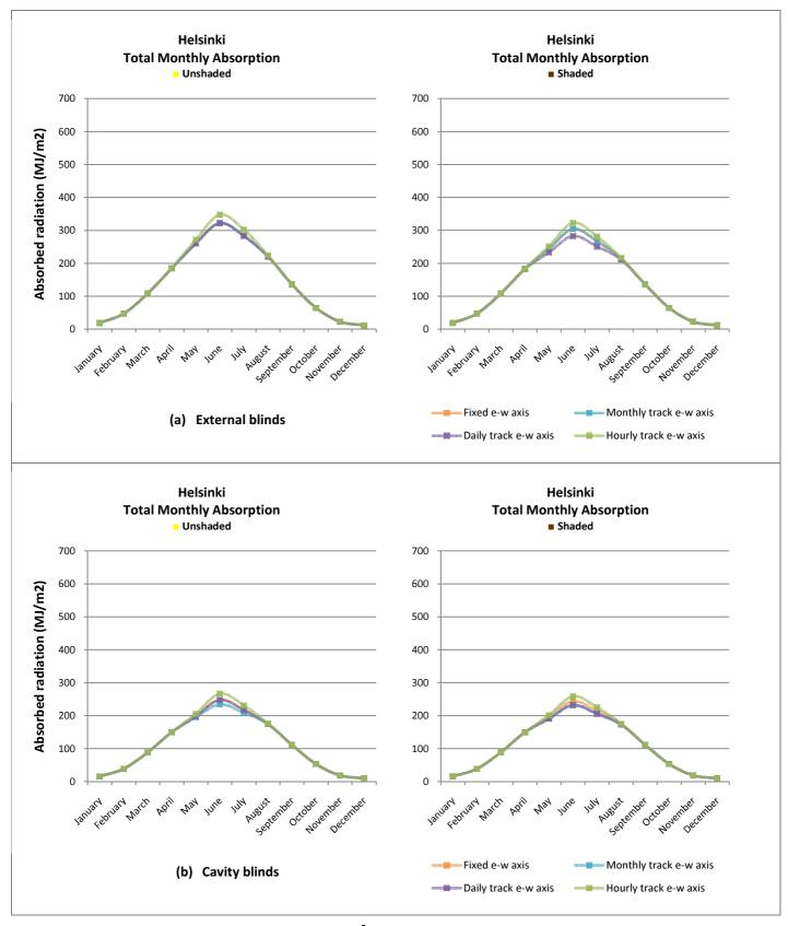
Figure 79. Absorption per m<sup>2</sup> of absorber surface for North Façade.
