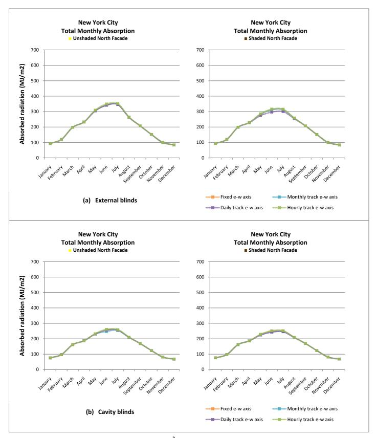
Figure 71. Absorption per m<sup>2</sup> of absorber surface for North Façade.
