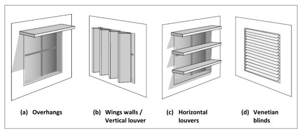
Figure 5. Different sun shading systems .
