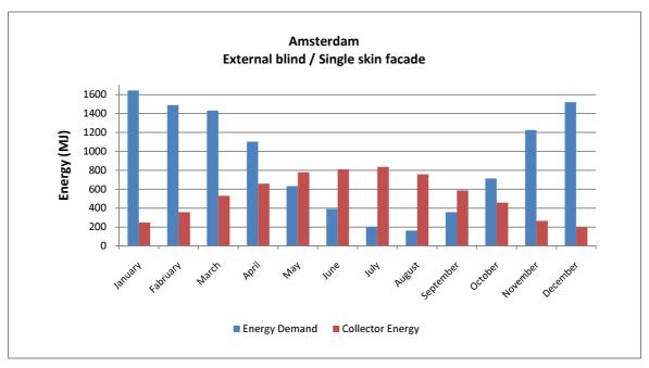
Figure 84. Energy demand and collector energy output for shaded cavity blinds.
