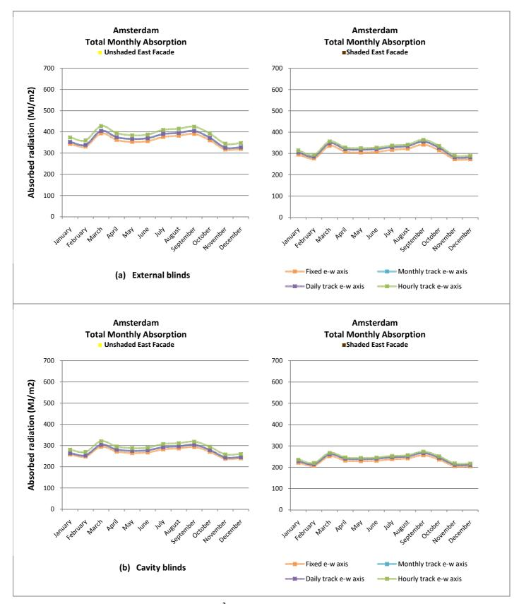
Figure 76. Absorption per m<sup>2</sup> of absorber surface for East and West Façade.
