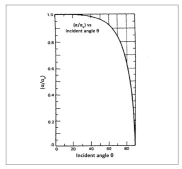
Figure 44. Ratio of solar absortance to solar absortance at normal incident for a flat black surface (Duffie, 2006).
