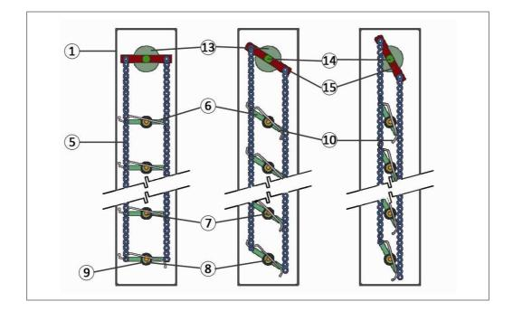
Figure 99. Principle of tilting mechanism for tracking blind.
