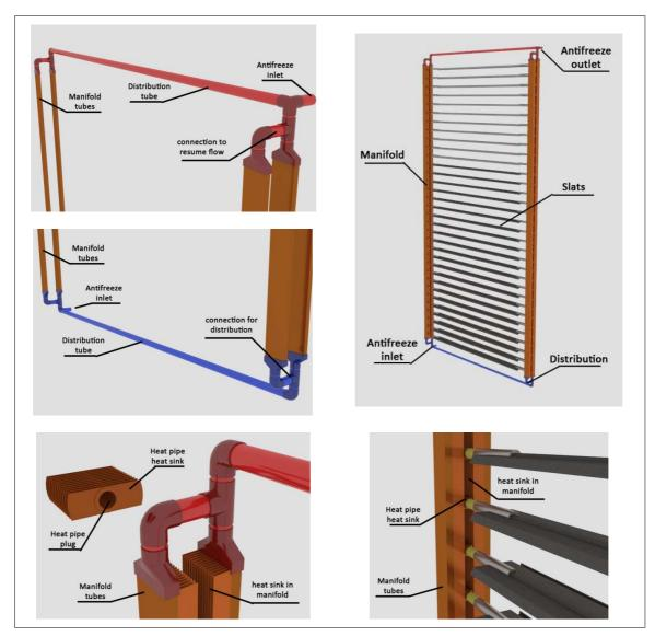
Figure 105. Manifold for retractable mechanism.
