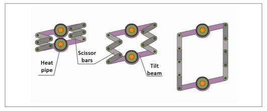
Figure 100. Scissor-like chain for tilting.
