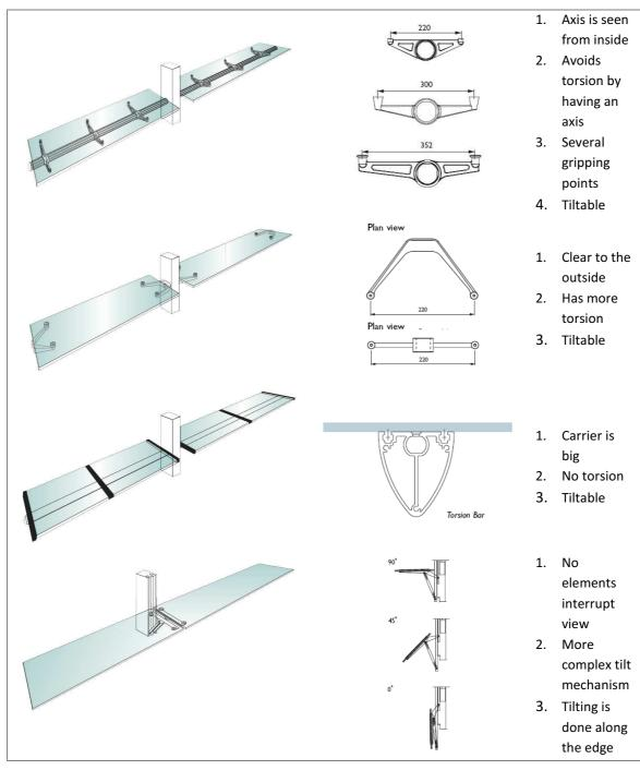
Figure 7. Louver carrier systems (Colt Int. Ltd., 2010).
