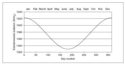
Figure 3. Variation of the extraterrestrial solar radiation throughout the year (Duffie, 2006).
