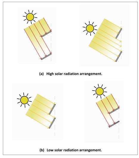
Figure 43. Offset of slats according to solar elevation.
