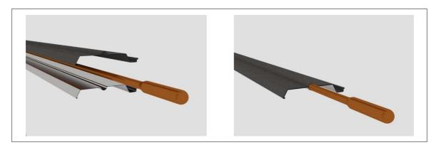
Figure 93. Slat and heat pipe connection.
