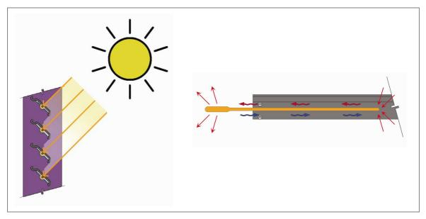
Figure 25. First part of the system: Collection of solar thermal energy through slats in a venetian blind.
