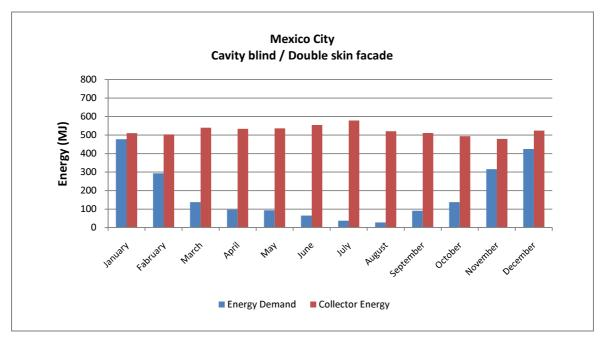
Figure 83. Energy demand and collector energy output for shaded cavity blinds.
