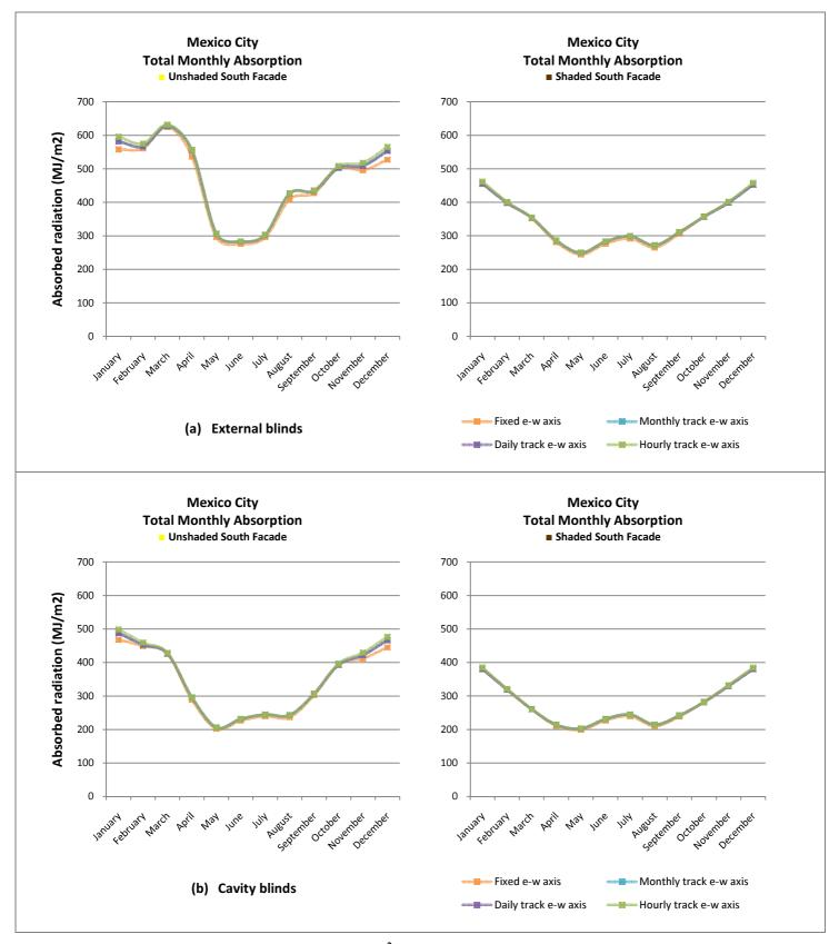
Figure 62. Absorption per m<sup>2</sup> of absorber surface for South Facade.
