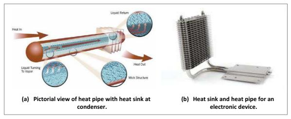
Figure 22. Heat pipe attached to heat sink. (Power Electronics Technology, 2011).
