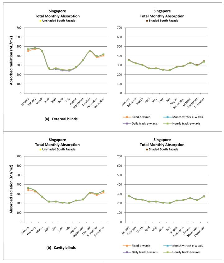
Figure 54. Absorption per m<sup>2</sup> of absorber surface for South Facade.
