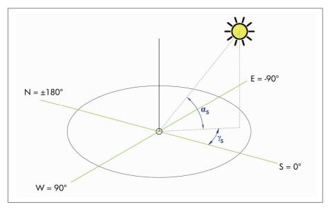
Figure 30. Solar altitude angle  $\alpha_s$  and Solar azimuth angle  $\gamma_s$ .
