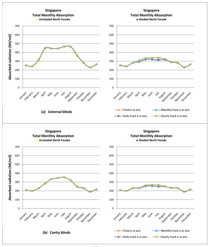
Figure 55. Absorption per m<sup>2</sup> of absorber surface for North Facade.
