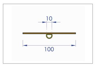
Figure 50. Contact area between slat and heat pipe.
