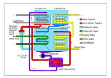
Figure 14. Absorption cooling system. (Encyclopedia of Alternative Energy and Sustainable Living, 2010)
