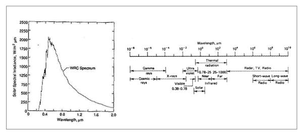
Figure 4. The WRC standard spectral irradiance curve at mean earth-sun distance (Duffie, 2006).
