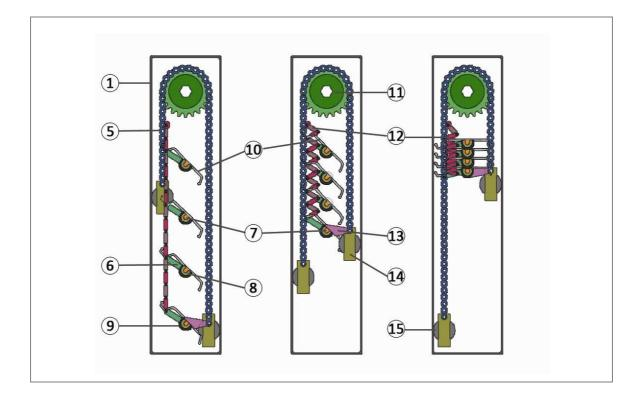
Figure 96. Principle of retracting mechanism for blinds.
