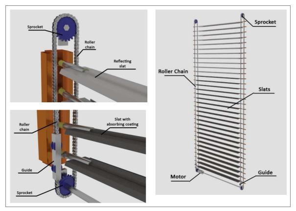
Figure 98. Retracting Mechanism.
