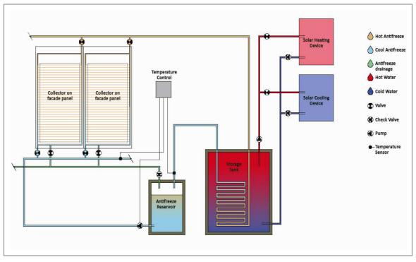
Figure 26. Solar thermal collection and cooling/heating systems interconnected.
