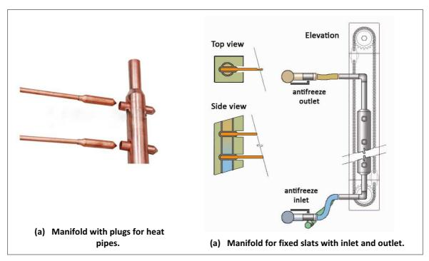
Figure 102. Principle of manifold for non-retractable blinds.
