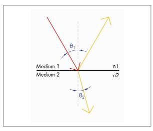
Figure 47. Incident and refraction angles for a ray that passes through different media.
