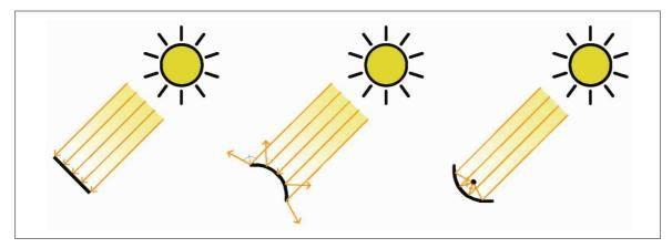
Figure 88. Three different shapes for a slat.
