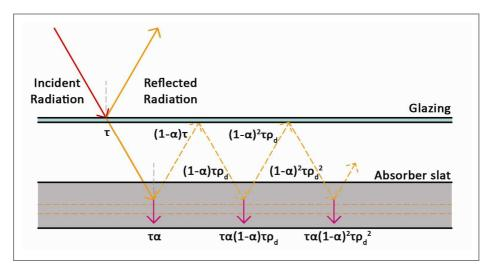
Figure 48. Top view of façade showing radiation transfer between glazing and absorber slats.
