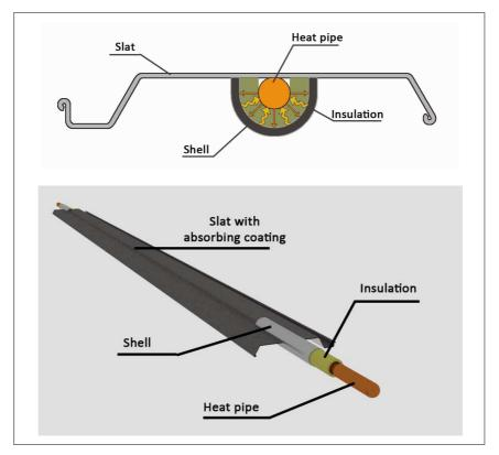
Figure 95. Coating on shell and reflection.
