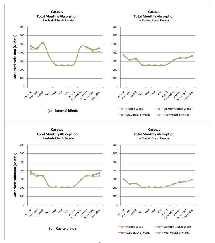
Figure 58. Absorption per m<sup>2</sup> of absorber surface for South Facade.
