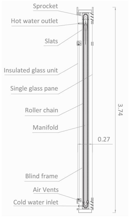
Plan 1. Vertical section of façade panel with solar thermal collector blind embedded.
