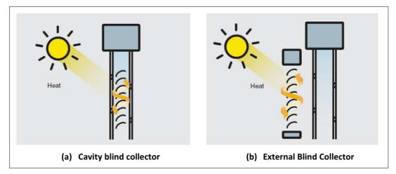
Figure 24. Blind collector placed inside the cavity and in front of the façade (Zumbotel, 2010).
