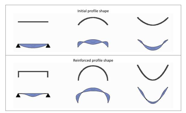
Figure 89. Reinforcement of slat profile shape for less torsion and deformation.
