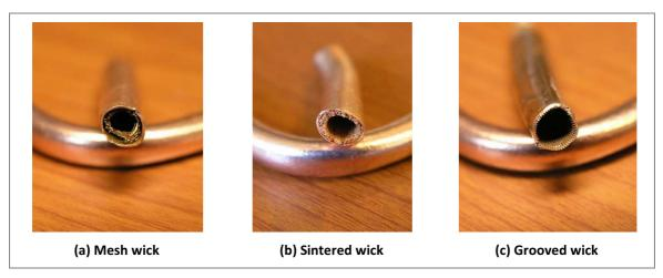
Figure 18. Different wick on heat pipes (Frosty Tech, 2010).
