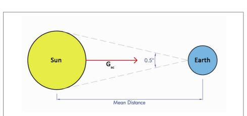
which is so minimal that the radiation emitted by the sun towards the earth results in a nearly fixed intensity of solar radiation outside the atmosphere of the earth (Figure 2).
