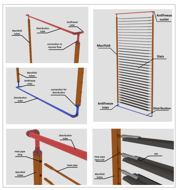
Figure 103. Manifold for fixed angle mechanism.
