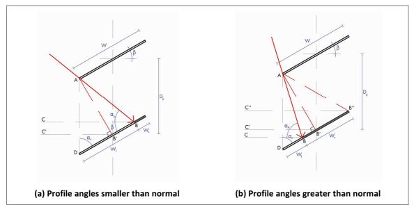
Figure 42. Geometry of shading on fixed slats.
