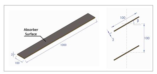
Figure 49. Slat geometry parameters for calculations input.
