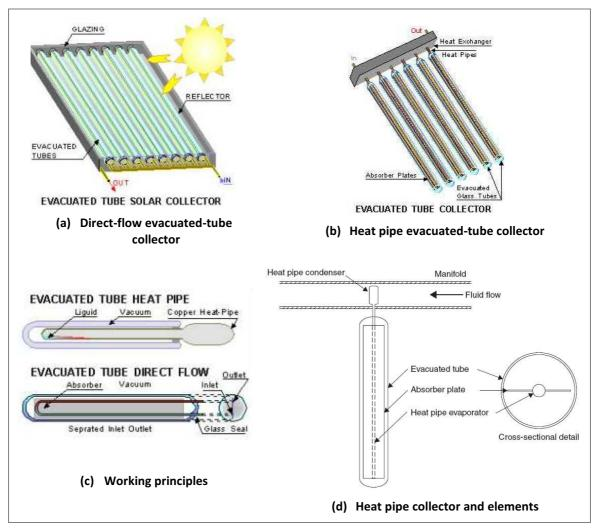
Figure 12. Evacuated-tube collectors and their elements (Encyclopedia of Alternative Energy and Sustainable Living, 2010).
