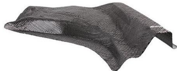
Figure 7.25 Carbon fibre preform for RTM production [61]
