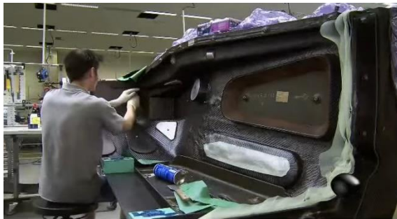
Figure 7.27 Lamination of mould segment of the Porsche 918 Spyder CFRP rear substructure [64]
