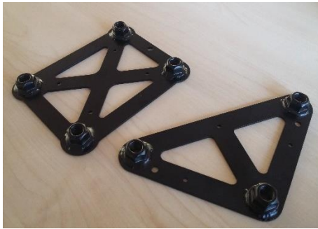
Figure 7.29 Nut plates as used in Roding Roadster
