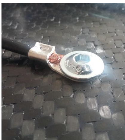
Figure 5.14 Connection of ground wire to rivnut, using an eyelet
