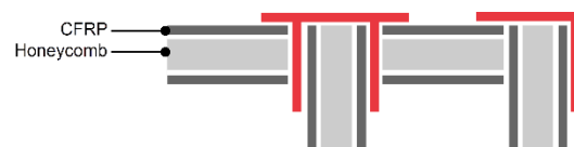
Figure 8.13 Covering profile for either corner joints or in continuing plates
