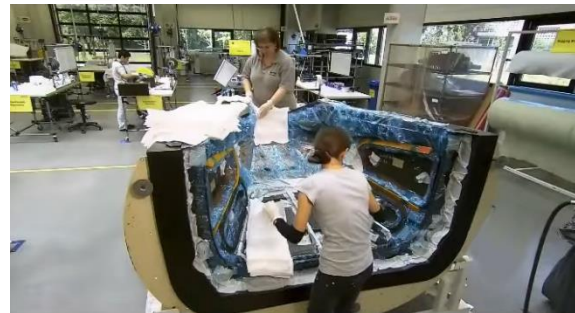
Figure 7.28 Combining the different mould segments and application of vacuum materials for the Porsche 918 Spyder rear substructure [64]
