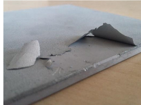
Figure 5.8 Zinc based EMI coating
