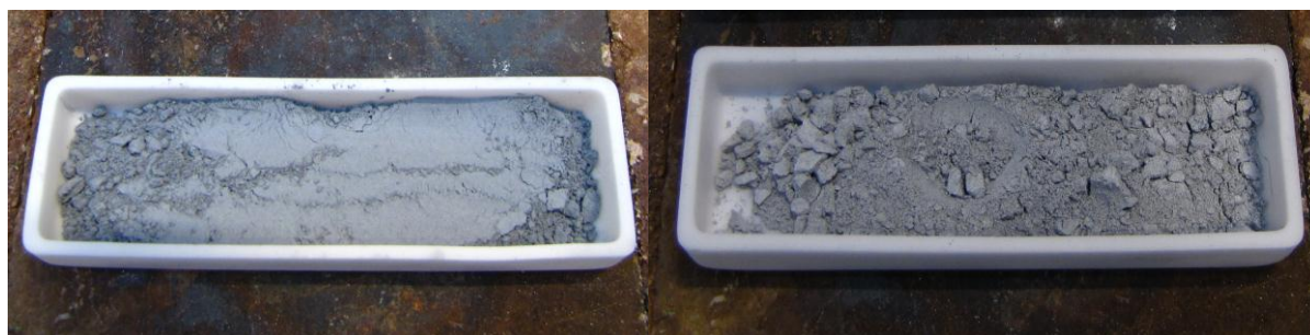
Figure 6.3 Photographs taken before (L) and after the experiment of G + C at 1300 °C.
