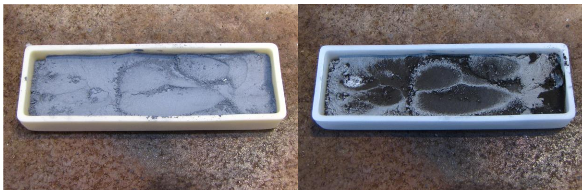
Figure 6.37 Photographs taken before (L) and after the experiment of G + Al at 1100 °C.
