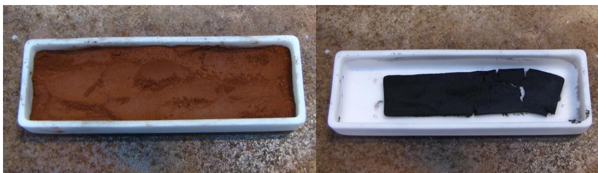
Figure 6.49 Photographs taken before (L) and after the experiment of G + F + C at 1300 °C.
