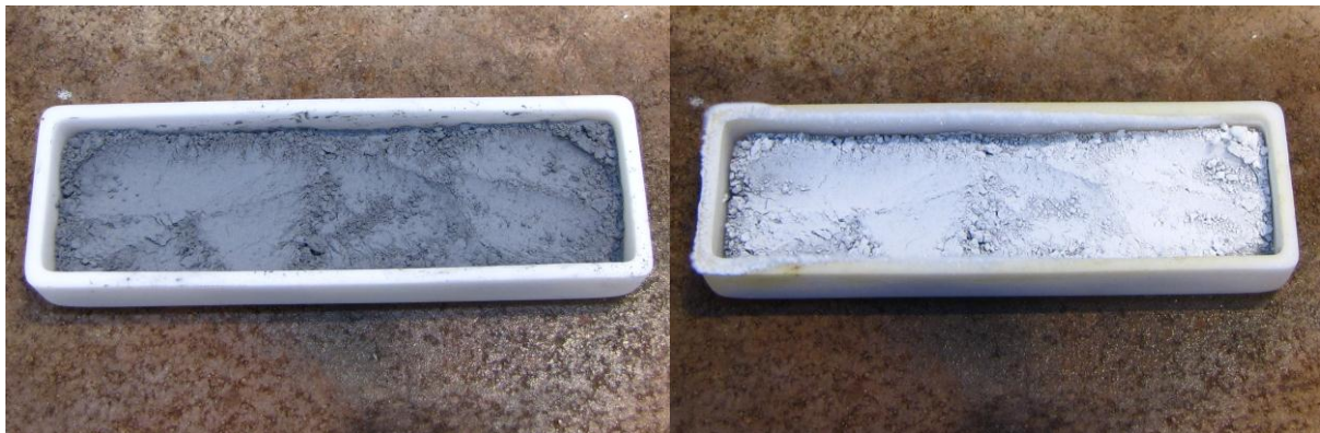
Figure 6.9 Photographs taken before (L) and after the experiment of G + C at 1200 °C.
