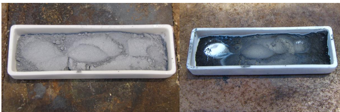
Figure 6.34 Photographs taken before (L) and after the experiment of G + Al at 1150 °C.
