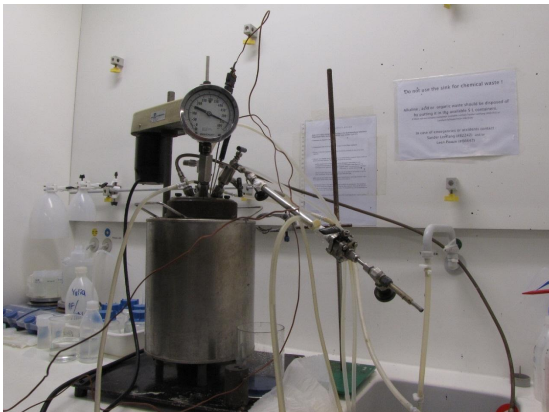
Figure 4.8 Autoclave featuring pressure meter, set of water cooling pipes, external thermocouple and sampling pipe.
