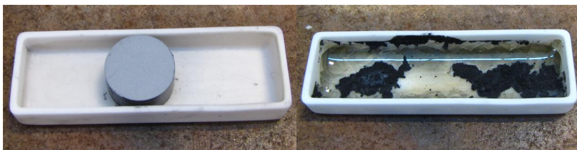
Figure 6.59 Photographs taken before (L) and after the experiment G + C + \text{SiO}_2 + \text{CaO} at 1400 °C.
