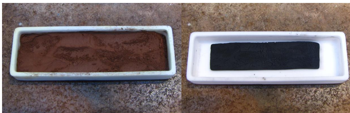
Figure 6.52 Photographs taken before (L) and after the experiment of \text{G} + \text{F} + \text{ZnO} + \text{C} at 1300 °C.
