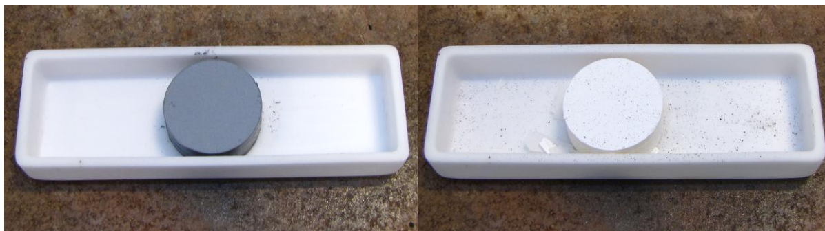
Figure 6.55 Photographs taken before (L) and after the experiment \text{G} + \text{C} + \text{SiO}_2 at 1200 °C.
