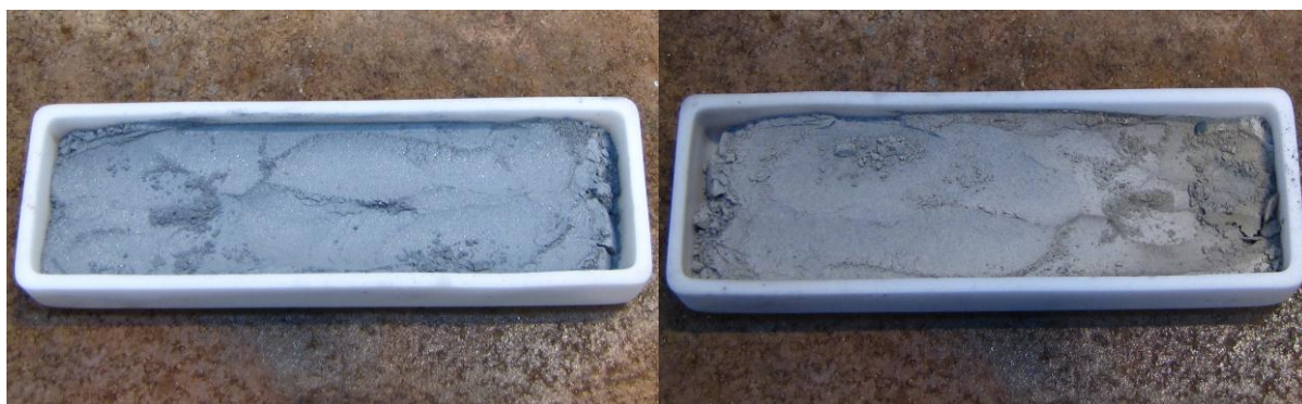
Figure 6.31 Photographs taken before (L) and after the experiment of G + Al at 1200 °C (powder).
