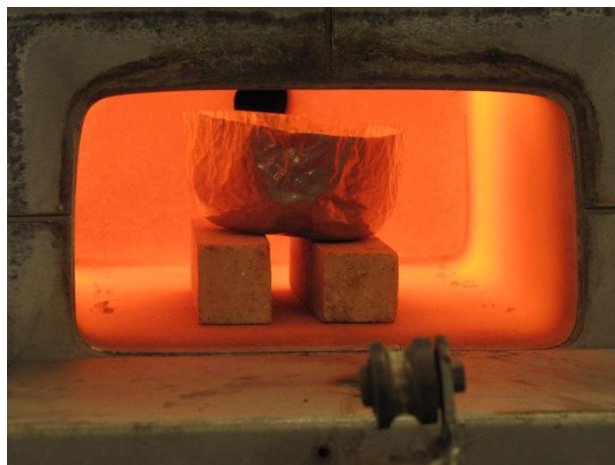
Figure 4.2 Heat treatment for gahnite synthesis (close-up at the platinum crucible).
