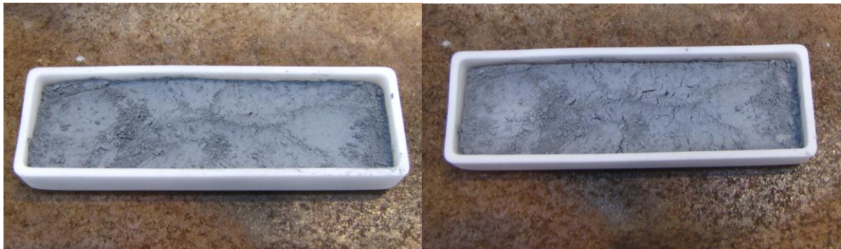
Figure 6.6 Photographs taken before (L) and after the experiment of G + C at 1250 °C.
