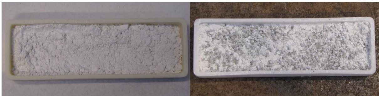
Figure 6.25 Photographs taken before (L) and after the experiment of G + Al at 1200 °C (balls).
