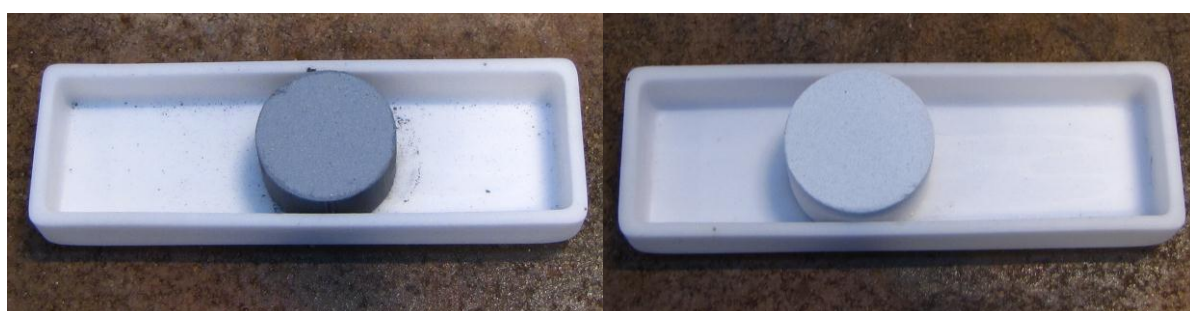
Figure 6.58 Photographs taken before (L) and after the experiment G + Al + SiO 2 at 1200 °C.
