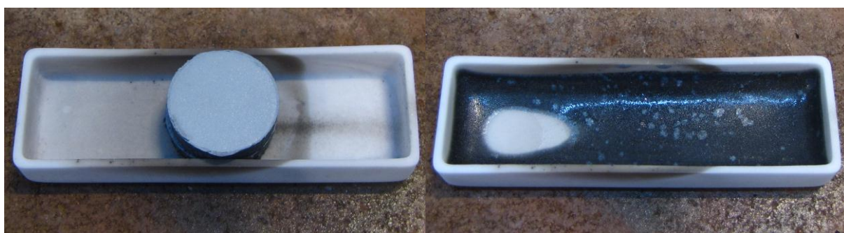
Figure 6.60 Photographs taken before (L) and after the experiment G + Al + SiO 2 + CaO at 1400 °C.
