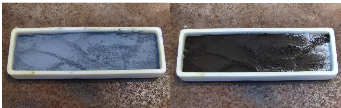
Figure 6.40 Photographs taken before (L) and after the experiment of G + Al at 1000 °C.
