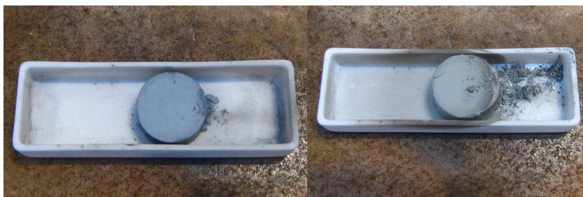
Figure 6.28 Photographs taken before (L) and after the experiment of G + Al at 1200 °C (tablet).
