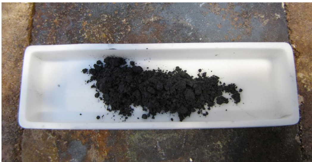
Figure 4.11 Pure carbon powder (graphite) utilized for the carbothermic reduction experiments.
