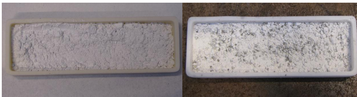
Figure 6.21 Photographs taken before (L) and after the experiment of G + Al at 1000 °C (balls).
