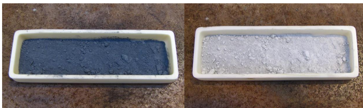
Figure 6.46 Photographs taken before (L) and after the experiment of G + Al at 900 °C.
