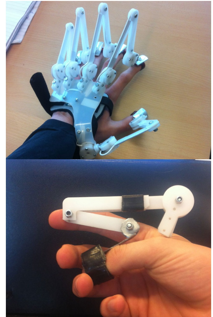
Figure 3.6 - Iterations of the Adjuvo Motion Sensor mechanism.
