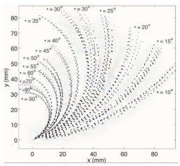
Figure 8. Positions of needle tips in the phantom. Insertion speed = 1,5 mm/s
