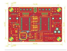
Figure 28. Dimensions of the PCB
