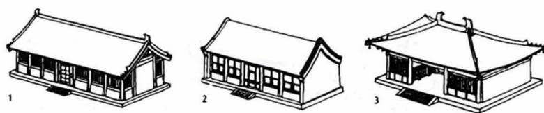
FIG. 4.18 The roof ridge changes from short to long (Sicheng Liang)
