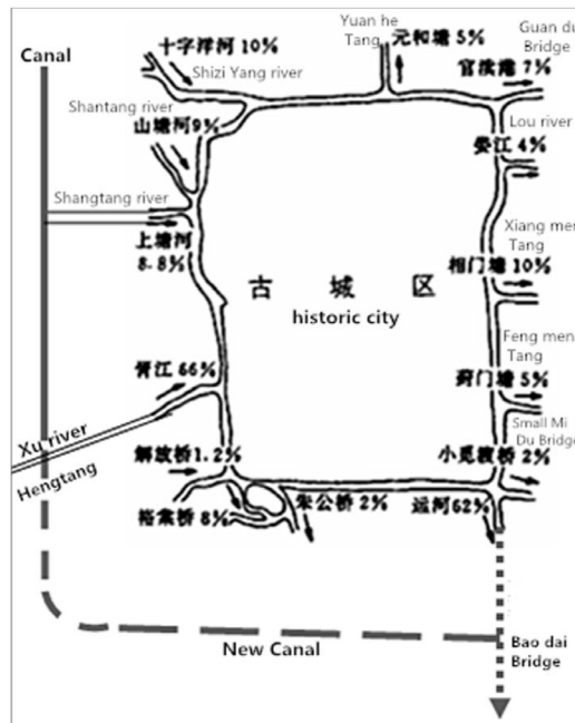
FIG. 4.37 Diagram of the third canal diversion project of Suzhou in 1992 (City Chronicle of Suzhou 1995)
