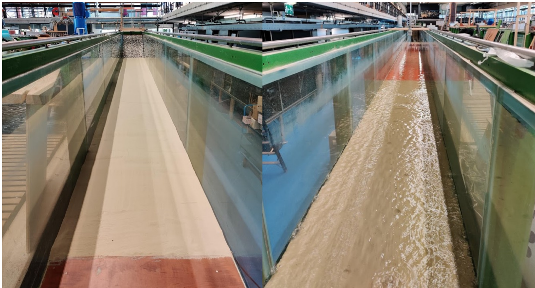
Figure 3.4: Sand pit facing structure (left) and sand pit and foreshore facing wave maker (right).
