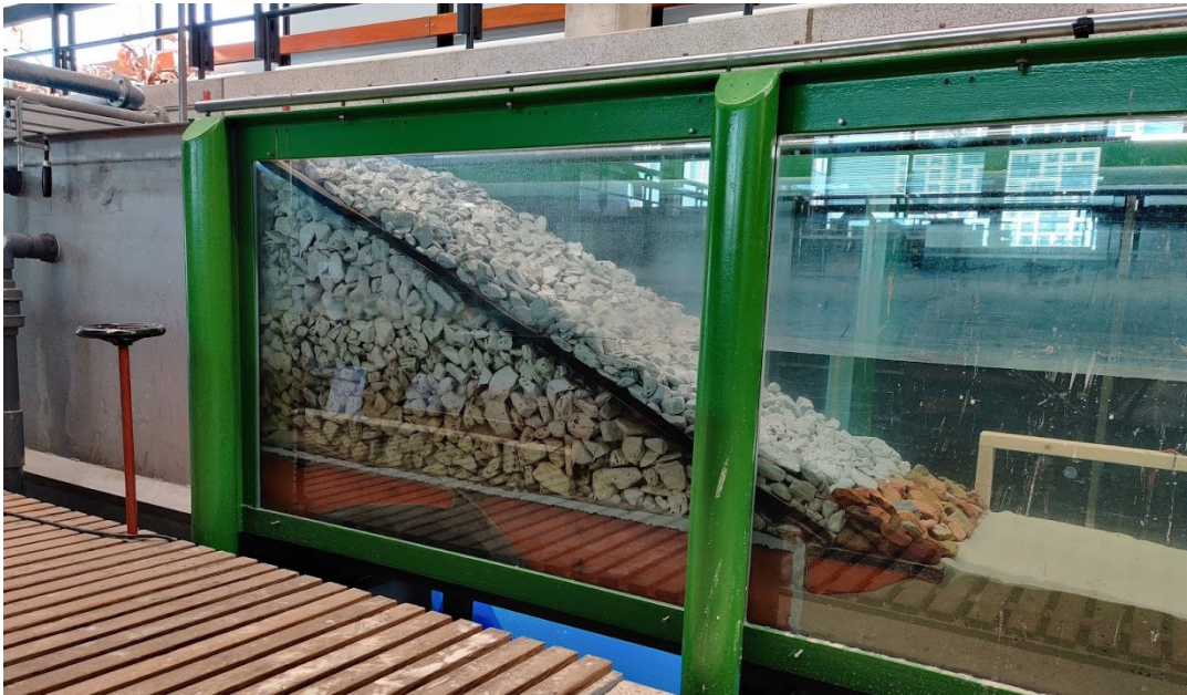
Figure 3.3: Revetment structure in wave flume, without toe and protection layer.
