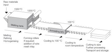
Figure 29. Float and rolled glass production process (Weller, 2009, P2-3)
