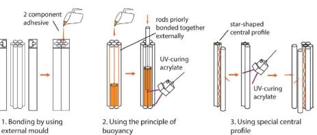
Figure 82. Illustration of the explored bonding techniques. Left: Bonding via the use of an external mould. Centre: Production technique using the principle of buoyancy. Right: Bundle with special central profile (Oikonomopoulou, 2016)
