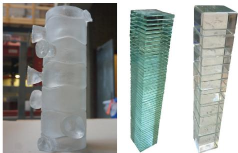
Figure 87. Left: Interlocking column of Akerboom (Akerboom, 2016). Right: Stacked float & cast glass column specimens (Felekou, 2016)
