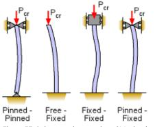
Figure 57. Column endconnections ('Mechanics eBook: Fixed Columns', n.d.)
