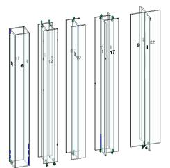
Figure 71. Revit model (3D) of the five configurations which shows the observed imperfections. The green arrows correspond to adifference in vertical position, the blue lines to an imperfection in the glue line and the small red figures to holes in the glass.(Ouwekerk, 2011)
