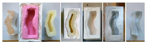
Figure 38. Production steps from MDF mould to final glass model of glass bridge components (Bristogianni et al, 2017 P1)
