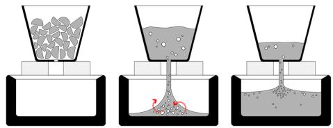
Figure 40. Air-entrapment during kiln-casting (Bristogianni et al, 2017, P27)
