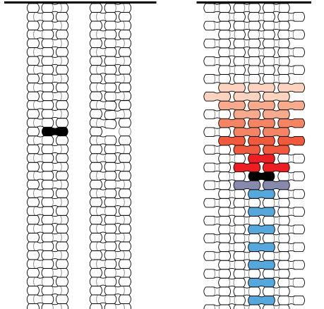
Figure 223. Block element breaks and the others will buckle a bit and take parts of the load
