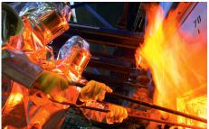
Figure 26. When producing float glass, temperatures exceeding 1,750 degrees Celsius are required - a challenge for both man and material. (Schott AG, 2014).jpg
