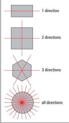
Figure 157. Optional interlocking shapes with their number of directions they could interlock
