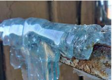
Figure 66. Melted glass after fire in building (Team WFM, 2011)
