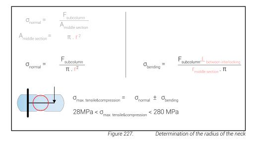
$\begin{array}{l} \boldsymbol{d}_{middle} = \left(2 \; . \; \boldsymbol{F}_{subcolumn} \; . \; \boldsymbol{L}_{interl} \; / \\ \left(\sigma_{maxtensileglass} \; . \; \boldsymbol{\pi}\right)^{1/3} \end{array}$
