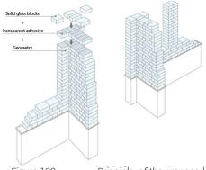
Figure 109. Principle of the proposed structural glass system (Oikonomopoulou et al., 2017)
