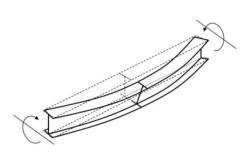
Figure 64. Torsional buckling schematicly ((Quora- Matmatch, n.d.)
