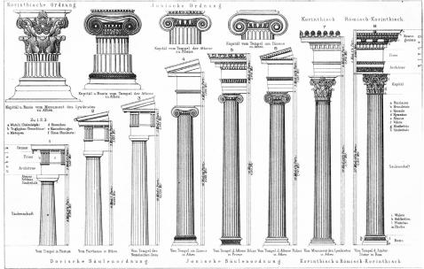
Figure 58. Illustration of Doric (left three), Ionic (middle three) and Corinthian (right two) columns.
