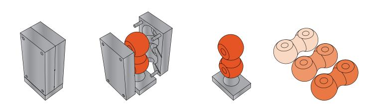
Figure 181. Steps in cast glass production with a pressuremould
