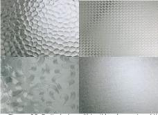
Figure 30. Rolled glass ('klasikbuzlucam', n.d.))
