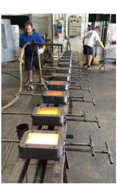
Figure 110. Molten glass bricks during the rapid cooling phase from 1200 to 700 degrees Celsius (Oikonomopoulou et al., 2017)
