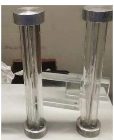
Figure 84. The 500 mm long specimen series tested in compression (Oikonomopoulou, 2017)
