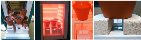
Figure 39. Kiln-casting method (Bristogianni et al,2017, P27)
