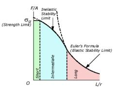
Figure 61. Graph with stress and Slenderness Ratio (eFunda, n.d.)
