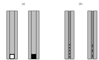
Figure 48. Cross-section of triple-layer annealed float glass beams with a stainless steel reinforcement section bonded at the inner recessed edge; (b) Cross-section of double-layer annealed float glass beams with GFRP reinforcement rods embedded in the interlayer. (Louter, 2011, P 253)
