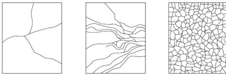
Figure 50. Schematic presentations (not to scale) of the fracture patterns of untreated and thermally, toughened glasses (Weller, 2009)
