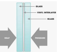
Figure 46. Laminating glass (Verrage, n.d.)
