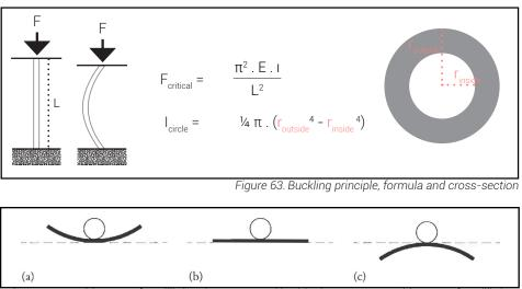
Figure 60. A stable state of equilibrium is represented by (a),whereas an unsrable state of equilibrium is represented by (c). The ball analogy for an indifferent state of equilibrium is shown in (b). (Roebroek, Snijder, Van Herwijnen, & Huveners, 2010)
