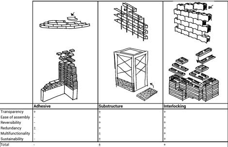
Table 7. Interlocking geometries with different structures (de Vries, 2018)
