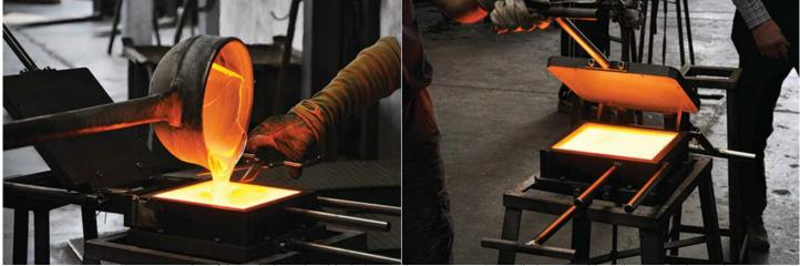
Figure 36. Casting of the soda-lime glass blocks by Poesia Company, using preliminary moulds. (Oikonomopoulou et al, 2014, P 209))
