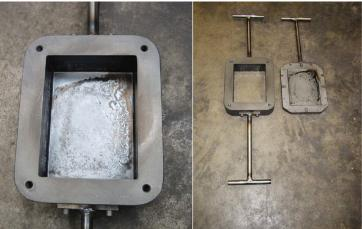
Figure 35. Final Precision moulds of soda-lime glass blocks (Oikonomopoulou et al, 2014, P 209)
