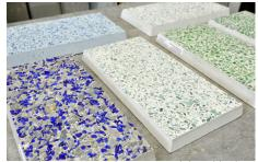
Figure 42. Sample concrete slabs with glass aggregates and different surface finishes (heringinternational, n.d.)
