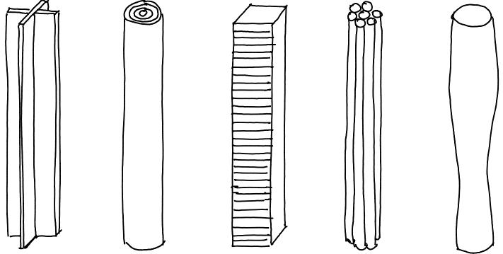
Figure 68. Types of glass columns : stacked , profiled, layered tubular, bundled, cast (Based on (Nijsse, R. & Ten Brincke, 2014), de Vries, 2018)
