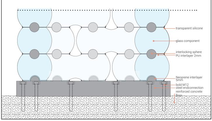
Figure 173. Detail of bottom part of the end-connection
