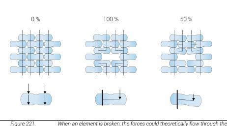
When an element is broken, the forces could theoretically flow through the elements above
