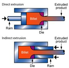
Figure 33. Extrusion process ('Granta's CES EduPack 2017', n.d.)
