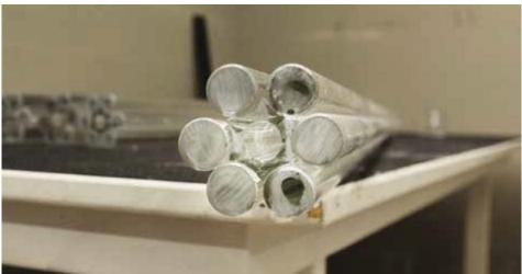
Figure 83. Rod configuration of the final bundled column design. (Oikonomopoulou, 2017)
