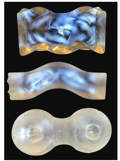
Figure 210. Stresses in the opper two components are much bigger then the lower one, due to the long annealing time and glass-like shape
