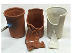
Figure 65. Thermal shock on ceramics ('The porcelain is harder, but the terra cotta has it beat for thermal shock!', n.d.)
