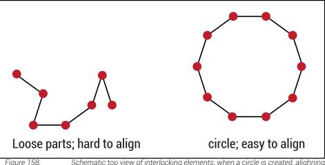
op view of interlocking elements: when a circle is created, alighning is easier.
