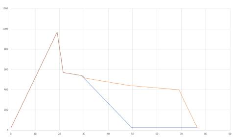
Figure 207. Diagram of firing schedule. Blue: the minimal annealing time for this glasstype and component. Orange: the annealing time the oven took, for the other components that were inside the oven.
