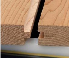
Figure 121. Toungue & groove (Retrieved from: http://www.woodworkersjournal.com/ cutting-tongue-groove-joints-table-saw/)
