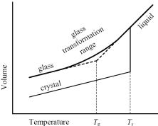
Figure 23. Schematic representation of volume's dependence on temperature for a glass and crystalline material ;Tg=glass transition temperature; Ts=melting temperature (Louter, 2011, P 46)
