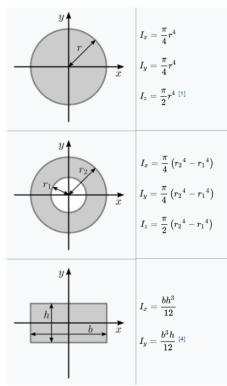
Figure 67. Second moment of area of different cross-sections (Circle, n.d., Rectangular area, n.d.)
