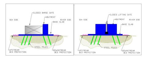
Figure 11- 2. Main gate objects (lift: barge gate; right: lifting gate)
