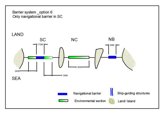
Figure 9-1. Schematic plan view of gate option
