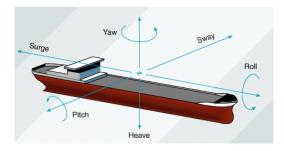
Figure 9- 30. Free floating structure motions modeled as a ship (Bennett Jr & Laborde, 2001)
