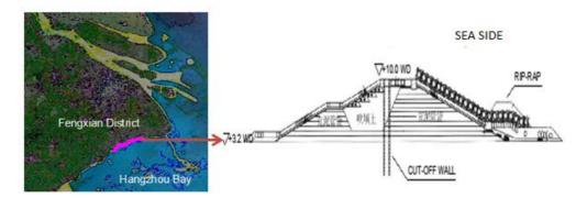
Figure A-1. Typical Cross Section of Sea Dike in Fengxian District
