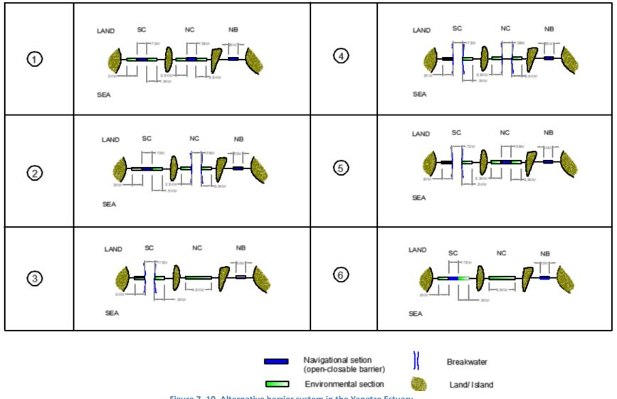
Figure 7- 10. Alternative barrier system in the Yangtze Estuary
