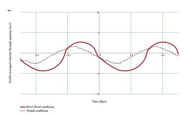
Figure 9- 40.Profile velocity through opening when all gates are opened (positive direction: from sea to the estuary)
