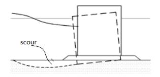
Figure 8-5. Scouring in front of a hydraulic structure
