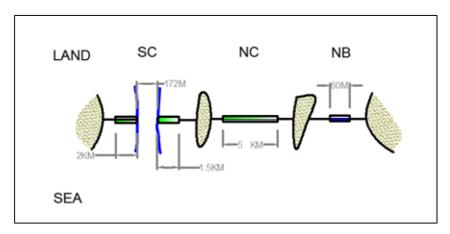
Figure K- 7. Plan view of open navigation channel option
