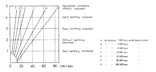
Figure 9- 38. Berthing gate velocity
