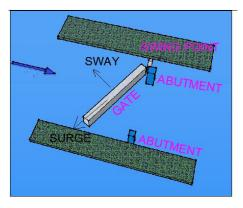
Figure 9-31. Restricted motions of floating gate during closure
