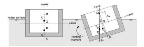
Figure 9-16. Metacentric height floating caisson (Erfeng Zhang et al., 2011)
