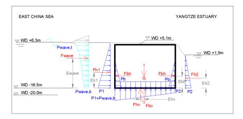
Figure 9-21. Force scheme of immersed gate due to hydraulic forces (storm condition)
