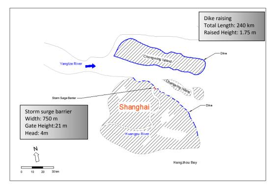
Figure 5- 6. Proposed Flood Defense System in Shanghai, Solution 2
