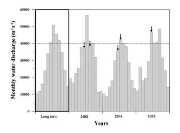
Figure 1- 3. Monthly water dishcharge rate (m<sup>3</sup>s<sup>-1</sup>) for long-term averaged values(in black frame) and for 2003, 2004 and 2005 at Datong Station, the seaward-most station of the Yangtze River. (Source: (Yang et al., 2006))
