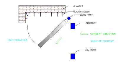
Figure 9-10. Plan view of floating gate after storm condition, not to scale
