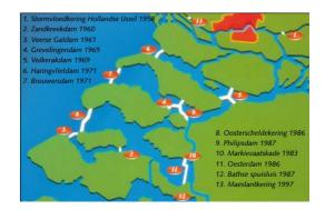
Figure 3-2. Present Storm Surge Barriers in the Delta Area (Source: (Rijkswaterstaat))
