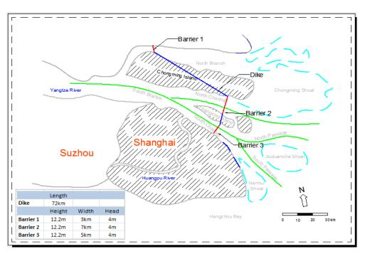
Figure 5-8. Proposed Flood Defense System in Shanghai, Solution 4
