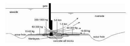
Figure 10- 5. Cross section bed protection of Maeslant barrier(Schiereck, 2001)
