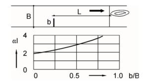
Figure 10- 12. Values for  $\alpha$  as a function of horizontal constriction for L/ $h_0$ =10
