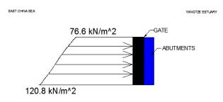
Figure 9- 24. Resultant distributed loads on the immersed gate when gate resting on abutments horizontally
