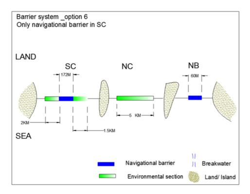
Figure K- 6. Barrier system option 6 – only navigational barrier in South Channel
