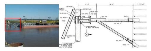
Figure 9-33. Articulation system of the Bayou Lafourche swing gate (Labeur, 2007)
