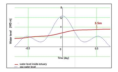
Figure 7- 13. Water levels inside the estuary in an open navigation section situation in design storm conditions (navigation channel width 375m)
