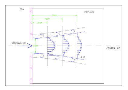
Figure 10-3. Velocity profile and influence of turbulence behind gap
