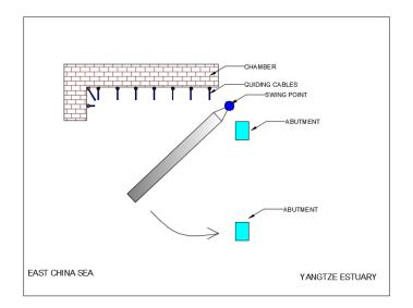
Figure 9-4. Bird view of floating gate during closing process, not to scale
