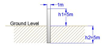
Figure E- 3. Typical Floodwall Cross Section Applied to Shanghai
