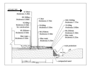
Figure 10-11. Designed bottom protection in the estuary side behind opening of open option
