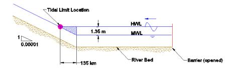
Figure 7-6. Indication of idealized tidal limit in the Yangtze River
