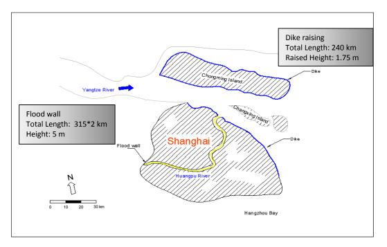
Figure 5-3. Proposed Flood Defense System in Shanghai, Solution 1
