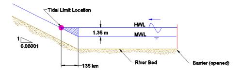
Figure H-1. Indication of idealized tidal limit in the Yangtze River
