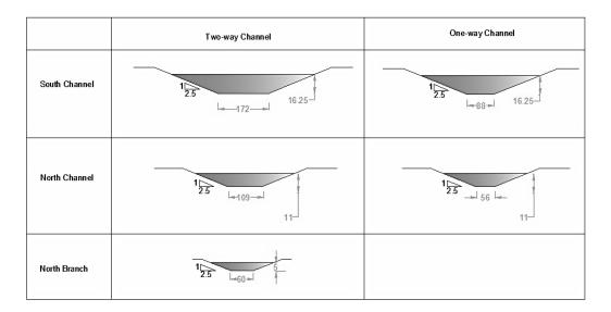
Figure 7-4. Proposed navigation channels cross sections
