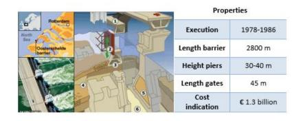
Figure 4-3. Eastern Scheldt Storm Surge Barrier and the Properties (Source: (de Gijt & van der Toorn, 2013))
