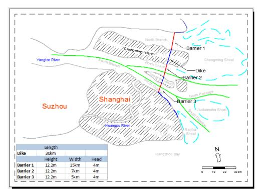
Figure 5-7. Proposed Flood Defense System in Shanghai, Solution 3
