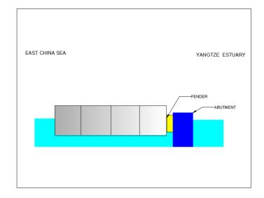
Figure 9-3. Side view of floating gate during closing process, not to scale
