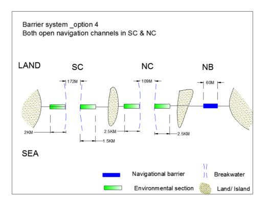
Figure K- 4. Barrier system option 4 – both open navigation channels in South Channel and North Channel
