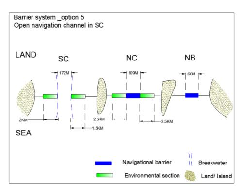
Figure K- 5. Barrier system option 5 – open navigation channel in South Channel
