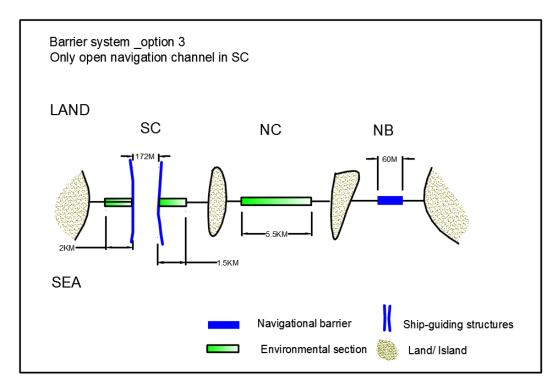
Figure 7-12. Schematic plan view of open option
