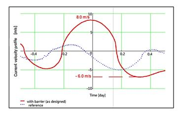
Figure 7- 14. Current velocity in the channel in open navigation channel option in design storm conditions (navigation channel width 375m)
