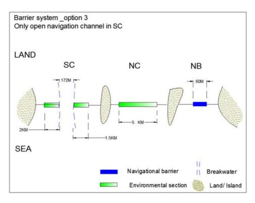
Figure K- 3. Barrier system option 3 – only open navigation channel in South Channel
