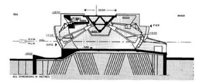
Figure 4-2. Cross Section of Haringvliet Sluice (Ferguson, Blokland, & Kuiper, 1970)
