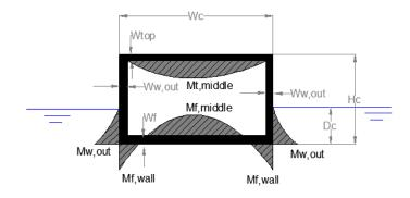
Figure 9-15. Moment scheme on a floating caisson
