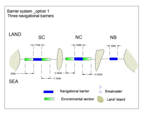
Figure K- 1. Barrier system option 1 – three navigational barriers
