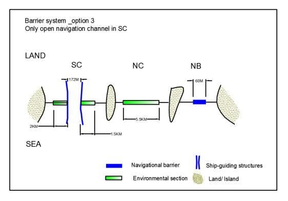
Figure 10-1. Schematic plan view of open option
