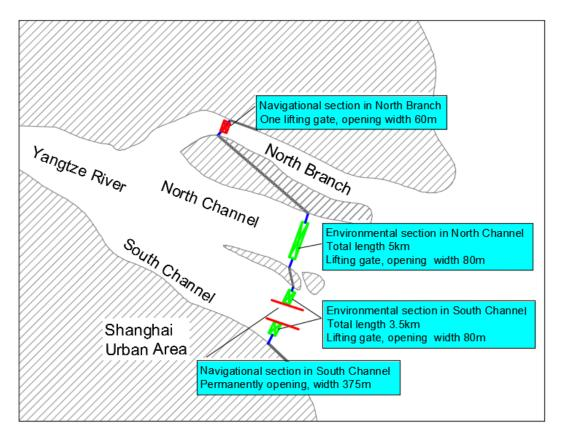
Figure 11-3. Overview of open option of barrier system in the Yangtze Estuary
