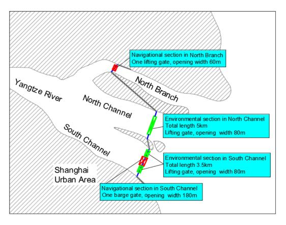
Figure 11-1. Overview of gate option of barrier system in the Yangtze Estuary
