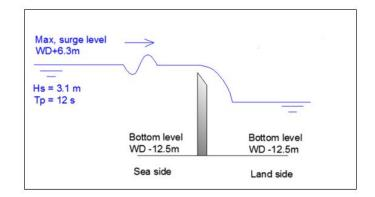
Figure 8-3. Modeled lifting gate and designed conditions
