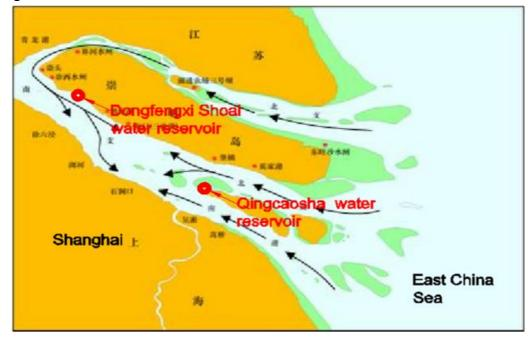
Figure G- 2. Salt Water Intrusion in the Yangtze River Estuary (Source: (Shanghai Water Resource Authourity, 2004))
