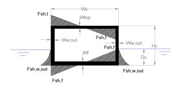
Figure 9-14. Shear stress scheme on a floating caisson
