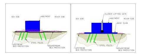
Figure 11-4. Main gate objects (lift: opening in South Channel; right: lifting gate)
