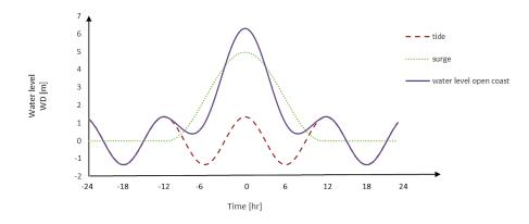
Figure 6- 2. Open estuary: water level for a 1/1,000 [1/year] design storm (data from Shanghai Water Authority)
