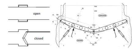
Figure C-1. Schematic Drawing of Mitre Gate with Basic Functional Principles
