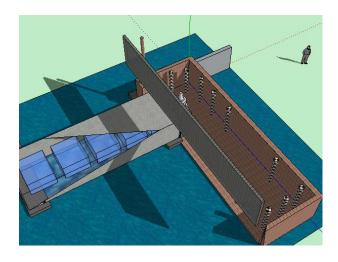
Figure 9-34. Designed dry chamber for barge gate when not in operation
