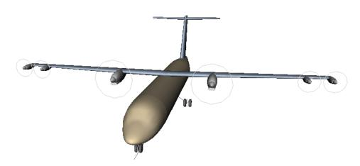
Figure 6.2: Series/parallel aircraft external propulsive system configuration.
