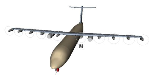
Figure 6.3: Series aircraft external propulsive system configuration.
