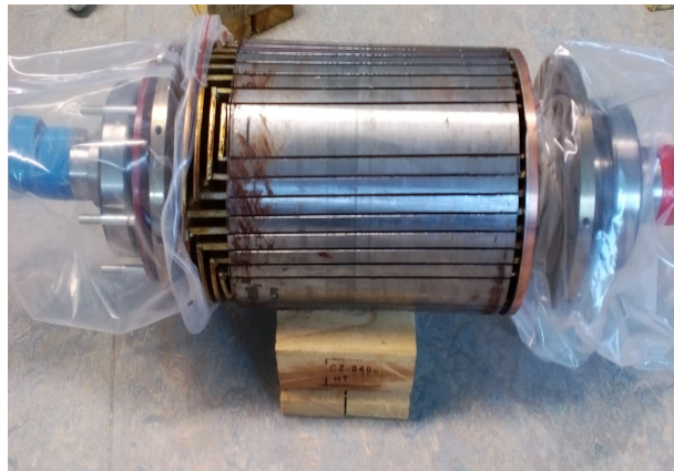
Figure 2.3: Skewed Nested cage rotor.
