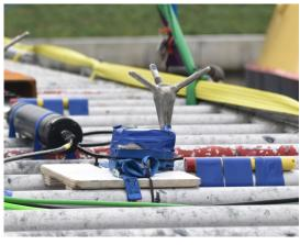
(b) Photo of ADV1 and RBR solo 1 illustrating how they are mounted on the horizontal measurement frame. The black band on the ADV arm in the centre of the photo indicates the positive x-direction of the ADV. On the left the case of the ADV can be seen which is placed just behind the location of the ADV head. On the right the RBR solo is taped to the scaffolding with the sensing element (red) pointed towards ADV1.
