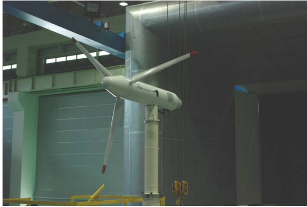
Figure 5.5: KARI wind tunnel with scaled down model of Mexico rotor, compare with figure 4.3
