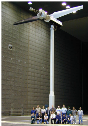
Figure 4.1: NREL Phase VI turbine in NASA Ames wind tunnel
