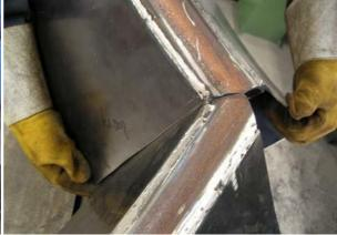
D. Positioning of two ribs of prototype 3.
