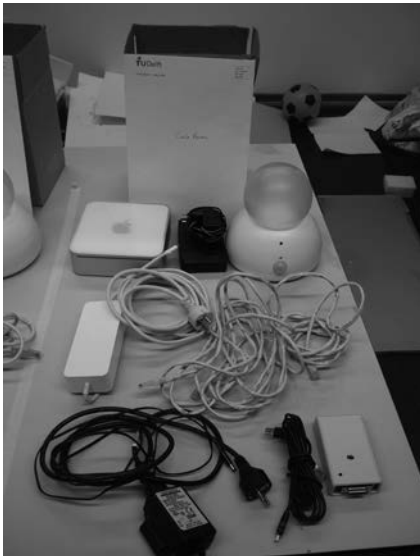
Figure 3.10. Hardware used in SnowGlobe field deployment, including adapters, network switch, Apple Mac Mini computer and SnowGlobe.
