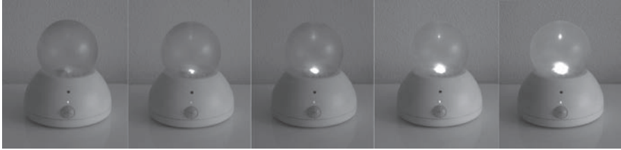
Figure 3.7. Brightness levels of SnowGlobe increasing from left to right: 0% - 25% - 50% - 75% - 100%.
