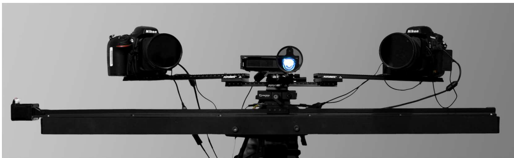
Figure 9-1: The imaging 'head' mounted on the linear ( x ) stage.
