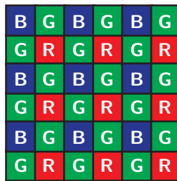
Figure 4-4: A Bayer filter of which each patch within the mosaic should be directly on top of one photosensitive element. This specific arrangement is called BGGR. Note there are twice as many green filters as there are blue and red, this is because the human eye (through evolution) is relatively more sensitive to green.
