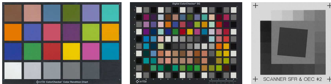
Figure 5-2: Three different targets used for camera calibration and performance benchmarking. Color-patch based targets (a) and (b) are industry standards used for color calibration and benchmarking, and target (c) is a slanted edge target that can be used for characterization of sharpness.
