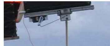
Fig. 1 Sliding mechanism along kite edge.
