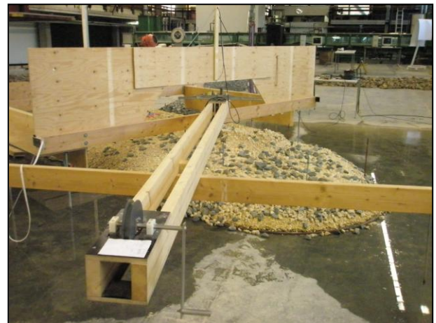
Figure 3.18: Measuring frame during measurement of the roundhead
