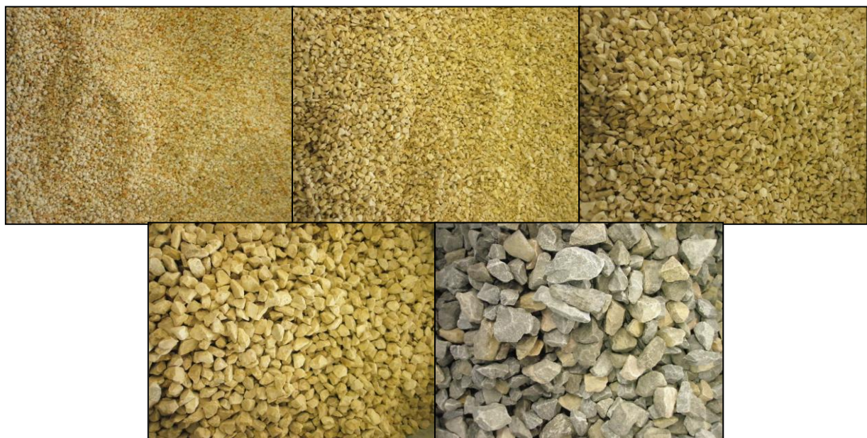
Figure 3.9: Samples of the five different fractions; 4-8mm, 8-11mm, 11-16mm, 20-40mm and 30-60mm
