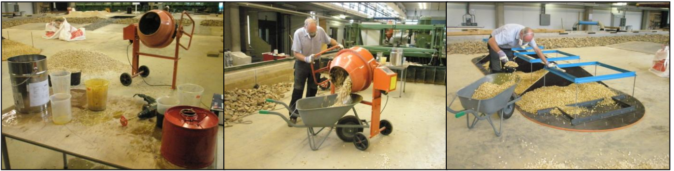
Figure 3.5: Process of mixing the stones with Elastocoast and application onto the model
