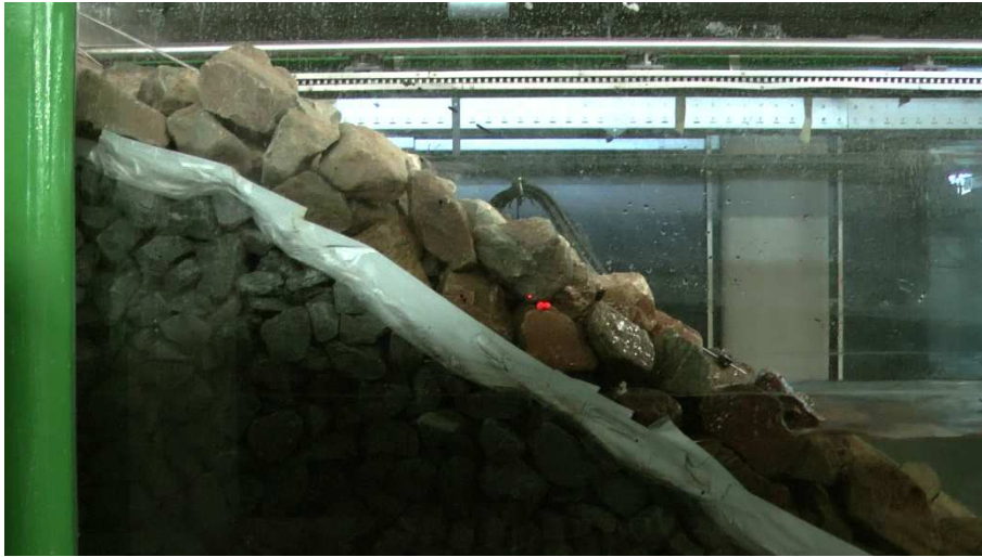
Photo 5: Side view of the armour layer on impermeable core
