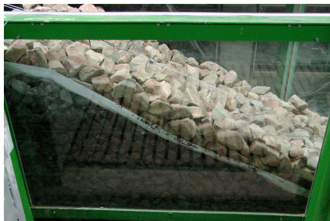
Photo 4: Side view armour layer on impermeable core, plastic sheet fixed at the sides by tape.
