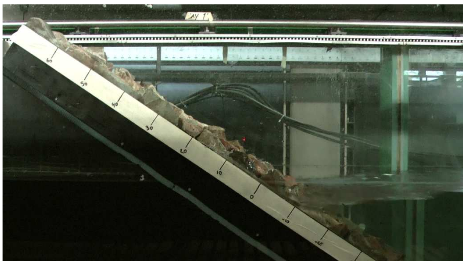
Photo 4: Side view of the rough impermeable slope 1:1.5
