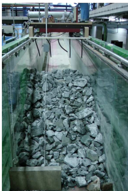
Photo 13: Building the core (grading 4)
