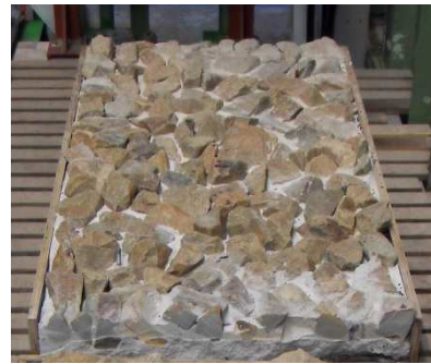
Photo 3: Rough impermeable slope (outside the flume)
