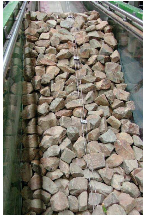
Photo 8: Armour layer with resistance wire on the slope
