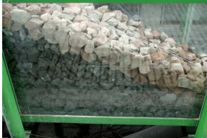
Photo 5: Armour layer on a permeable core, with a grading of 4
