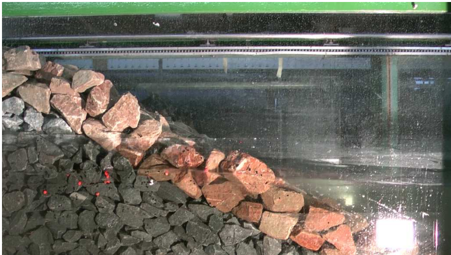
Photo 6: Side view of an armour layer on permeable core
