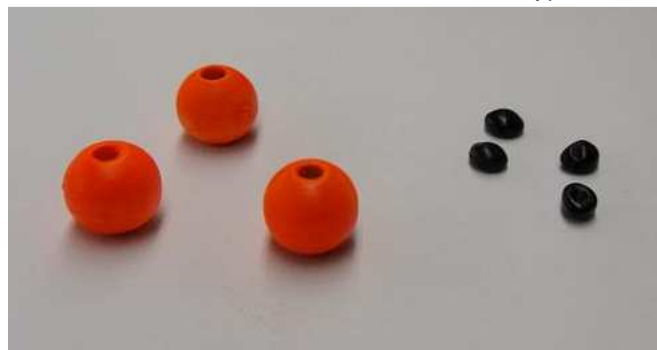
Photo 1: Left red wooden tracers 8 mm and right plastic tracers
