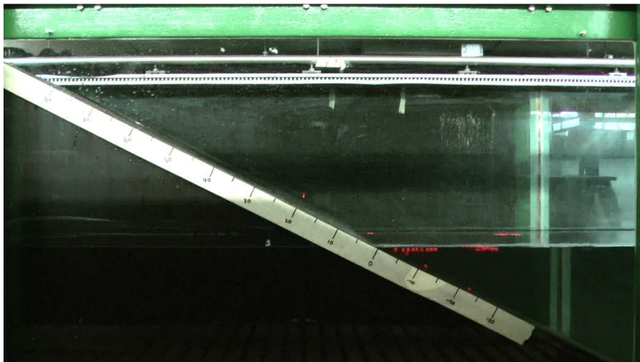
Photo 3: Side view image of the smooth slope 1:1.5
