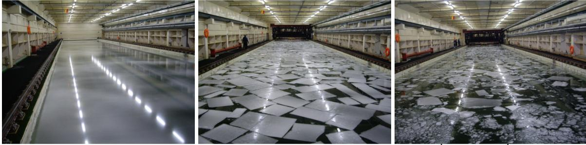
Figure 1. Ice concentrations in the ice tank: level ice, 8/10<sup>th</sup> and 6/10<sup>th</sup>.
