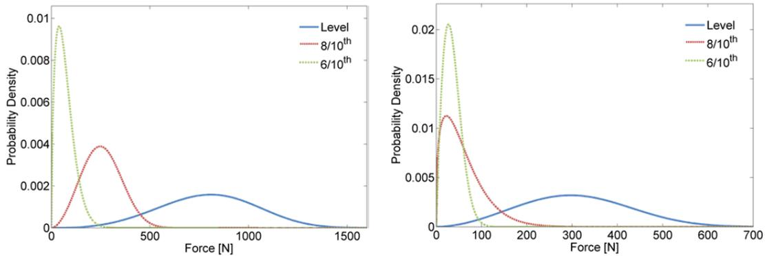
Figure 6. PDFs for 33 mm ice thickness,  $22.5^\circ$  orientation, a) full structure. b) design leg.
