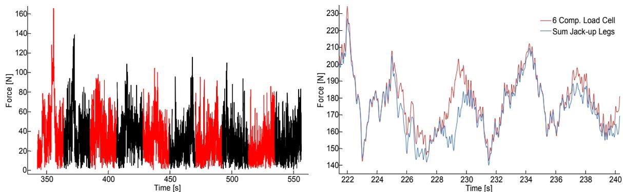
Figure 4. a) The resultant load on a front leg for test-run 11012 divided in 10 segments.
