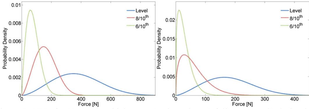
Figure 5. PDFs for 33 mm ice thickness,  $0^\circ$  orientation, a) full structure. b) design leg.
