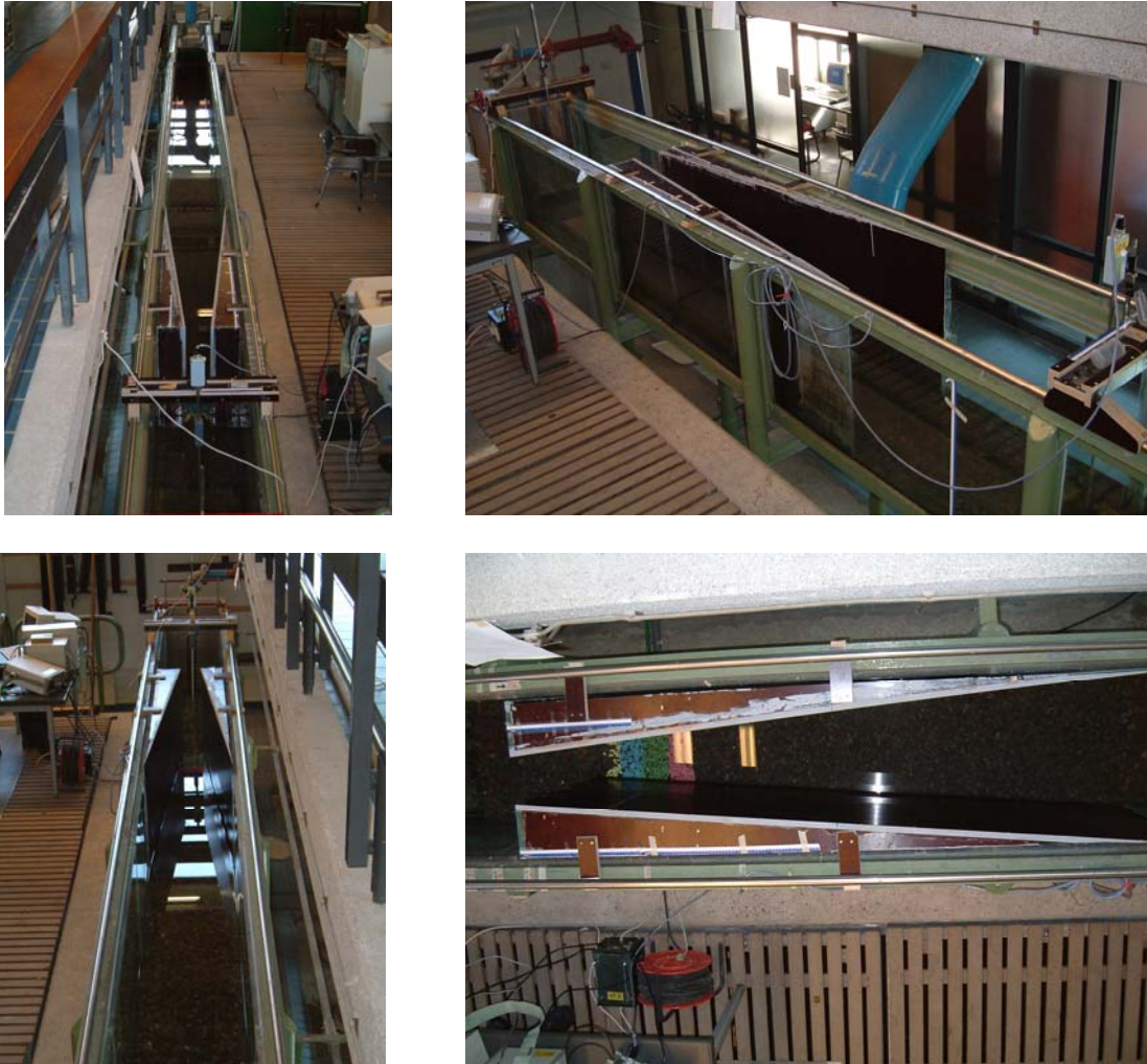
Figure A.1 The flume with a tapered section near the end
