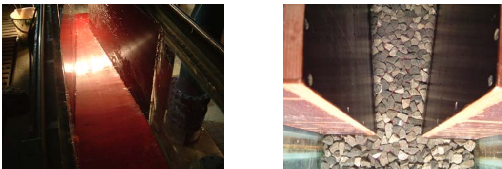
Figure A.2 The first layer of stones glued to the wooden bottom plates
