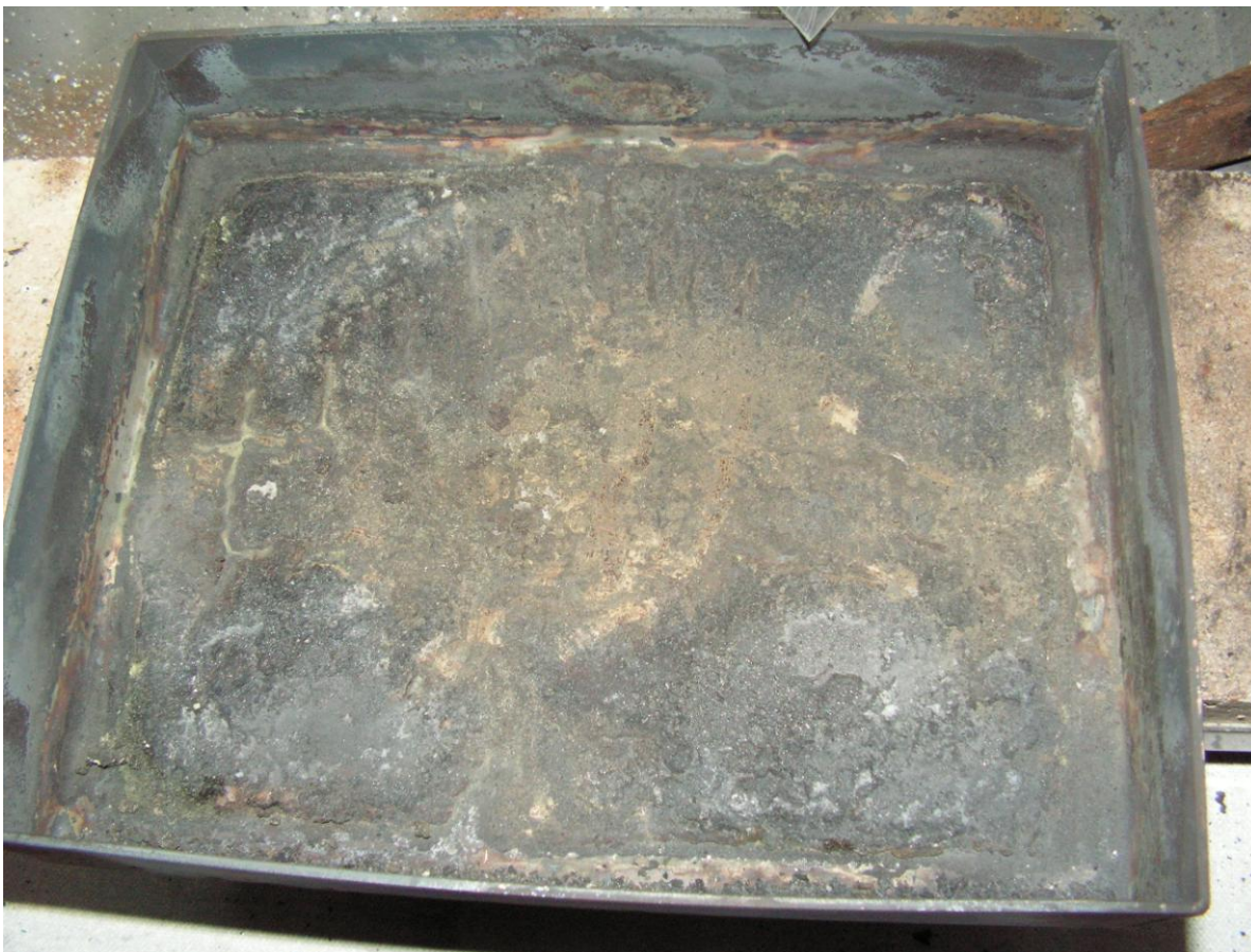
Figure 45. Corrosion effect of tray after roasting Zinc A with \text{Na}_2\text{CO}_3 .
