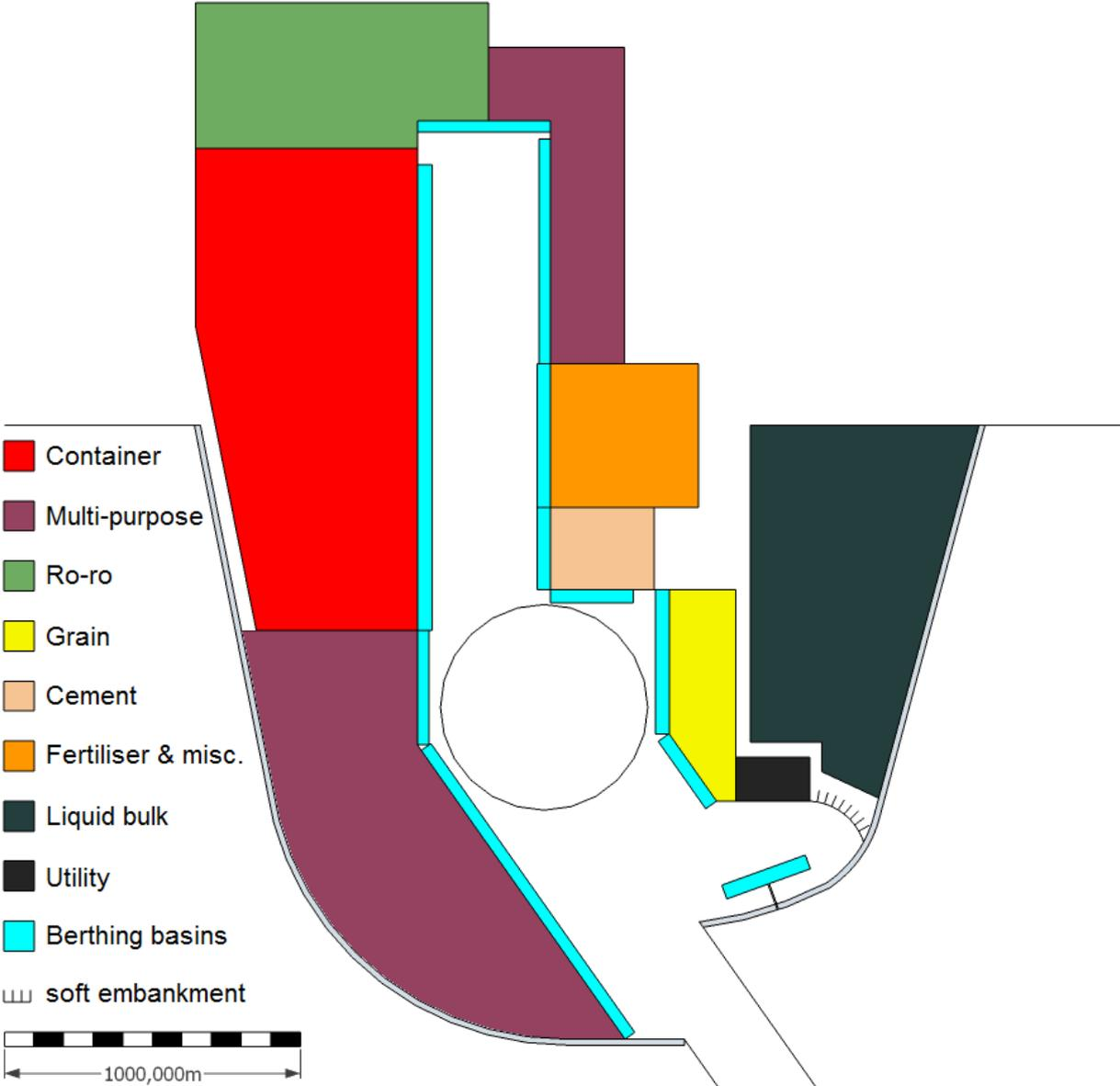
figure 35: Final layout. Dimensions are omitted for simplicity, they can be found in the following subparagraphs.
