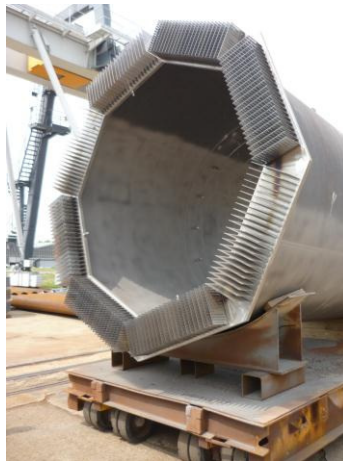
Figure K-9: The connection between tower and adapter is also made with perforated steel plates
