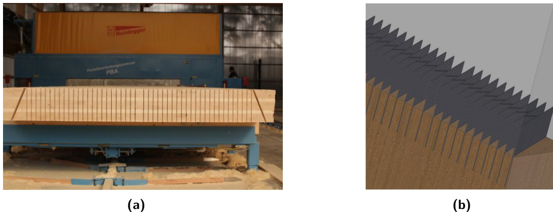
Figure 4-4: Horizontal connections are made by steel plates inserted into slots in the bottom and top edge of the panels
