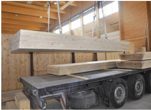
(a) The panels fit on a standard-sized truck Source: TimberTower GmbH, http://timbertower.de , accessed December 2013
