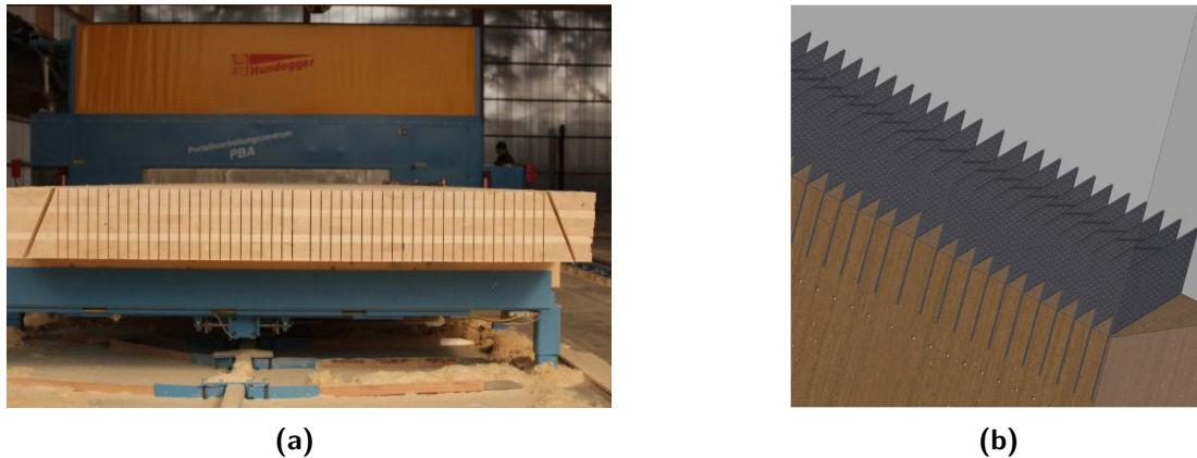
Figure K-7: Horizontal connections are made by steel plates inserted into slots in the bottom and top edge of the panels
