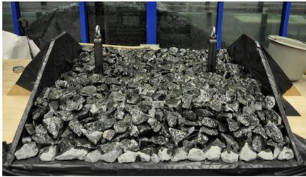
(c) First layers of stones fixed with epoxy
