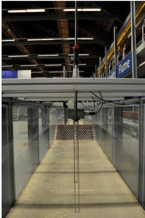
(a) Position wave height meter in cross-section
