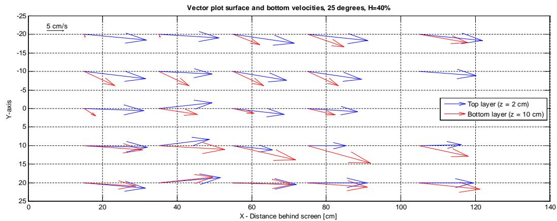
Figure 56 Top view velocity vectors behind the screen
