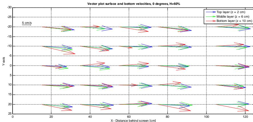
Figure 16 Top view velocity vectors behind the screen, 3 layers
