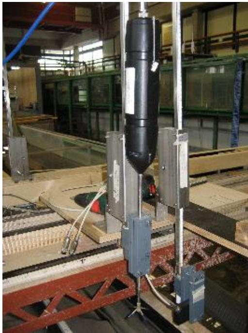
Figure 7 Vectrino mounted on measuring chart
