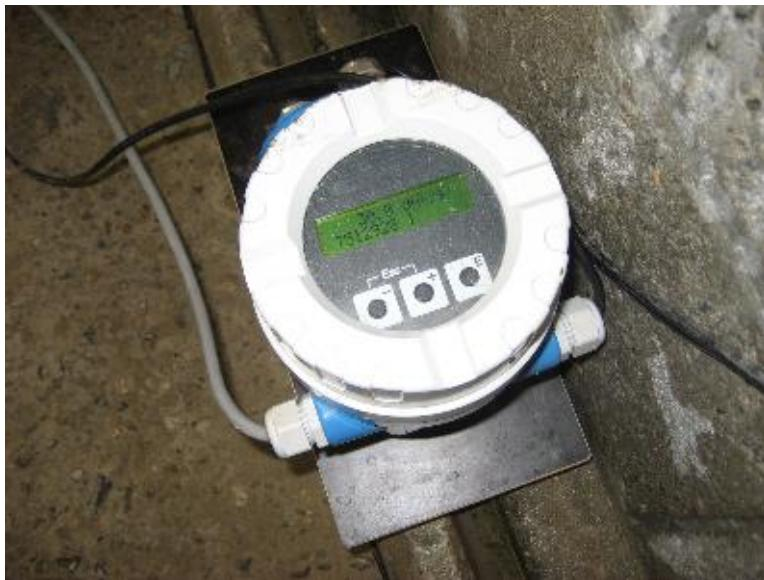
Figure 9 Display of discharge measurement device
