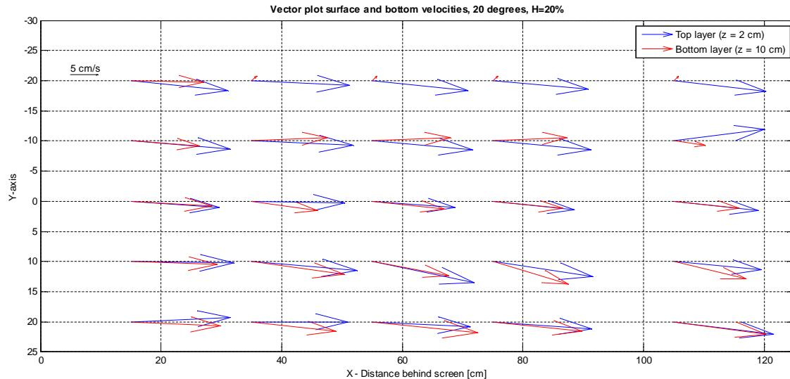
Figure 26 Top view velocity vectors behind the screen
