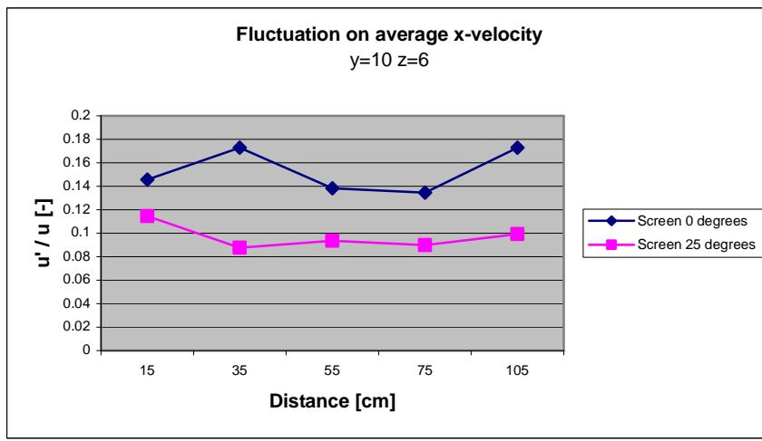
Figure 64 Turbulence different angles,  $y=10, z=6$
