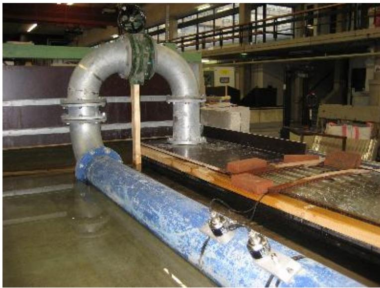
Figure 10 Acoustic sensors of the Proline Prosonic
