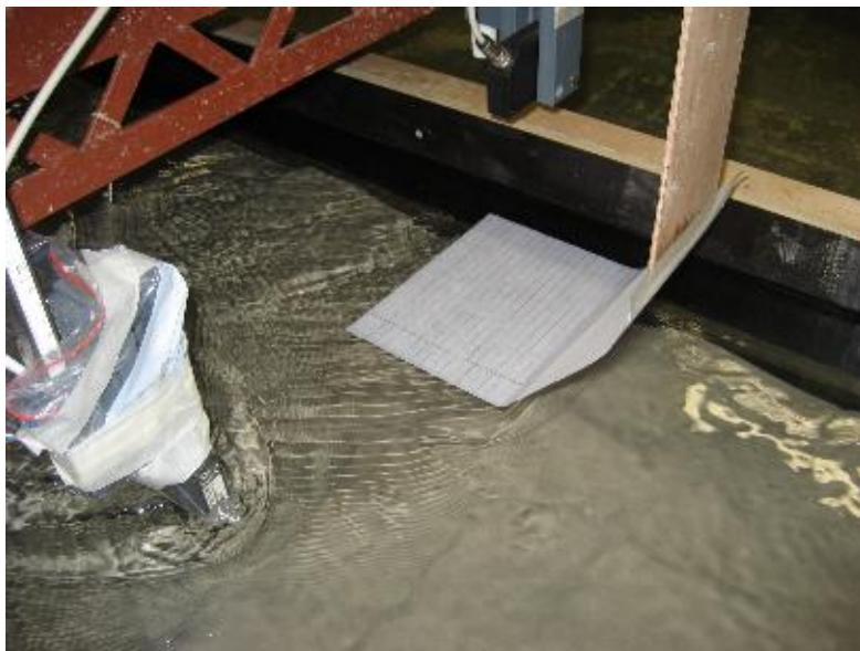
Figure 14 Lasers for water level and bed level measurement
