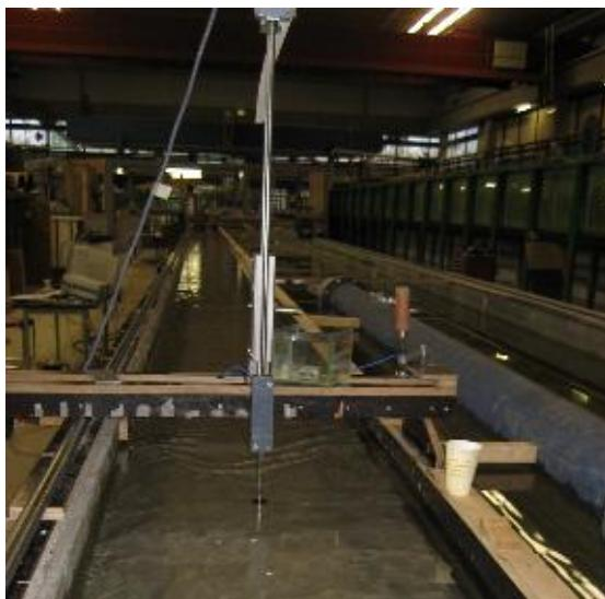
Figure 8 The EMS velocity measurement device
