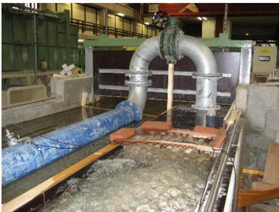
Figure 4 Upstream boundary condition in front of perforated plate
