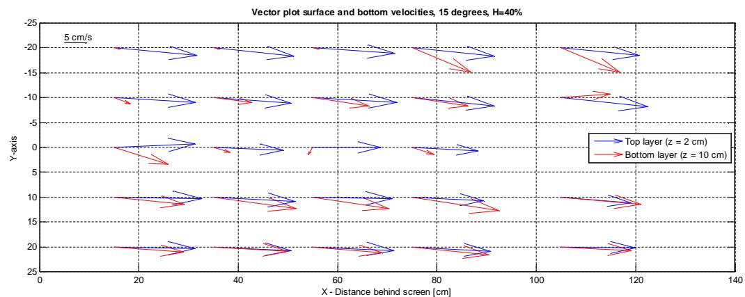
Figure 44 Top view velocity vectors behind the screen
