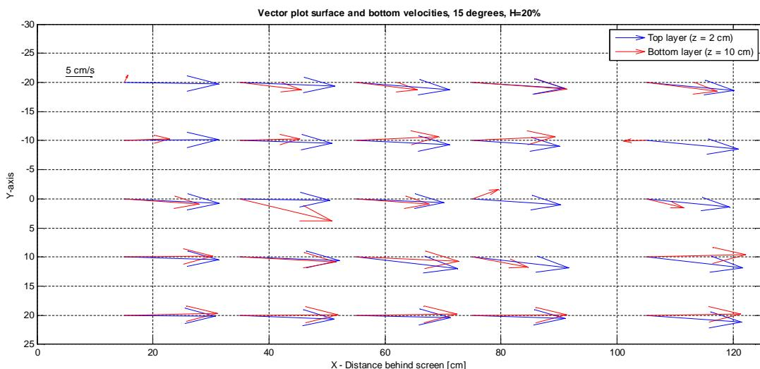
Figure 18 Top view velocity vectors behind the screen
