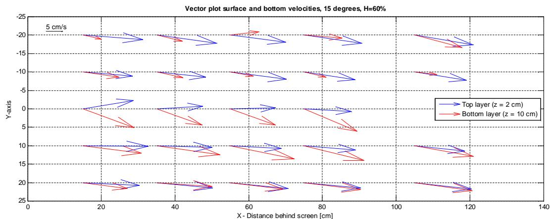
Figure 47 Top view velocity vectors behind the screen
