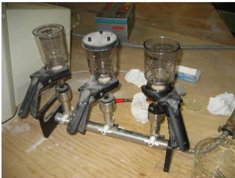
Figure 13 Vacuum filter for separating the water-sediment mixture
