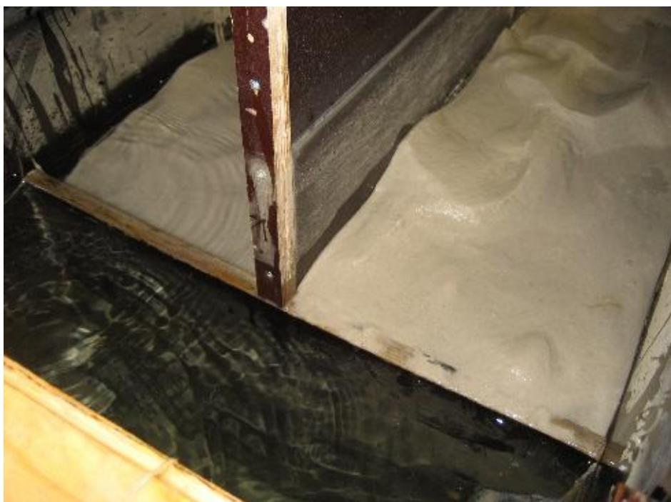
Figure 6 Sediment weir on bed level at the downstream boundary
