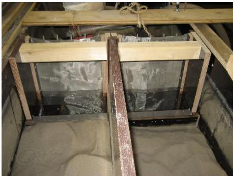
Figure 12 Sediment trap at the downstream boundary
