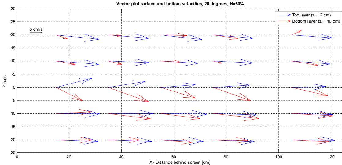
Figure 32 Top view velocity vectors behind the screen
