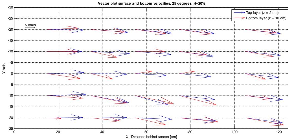
Figure 35 Top view velocity vectors behind the screen
