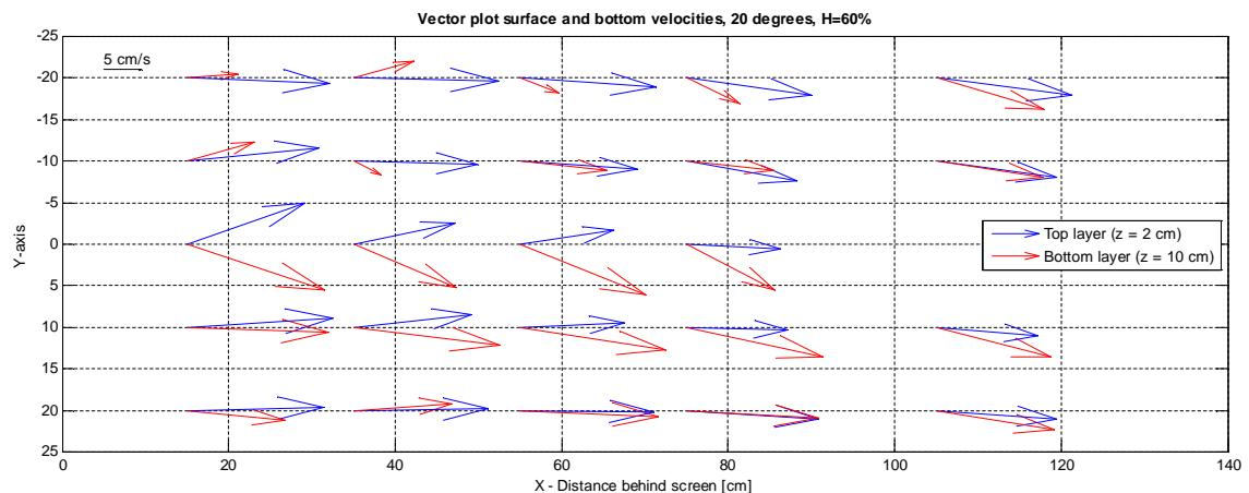
Figure 53 Top view velocity vectors behind the screen
