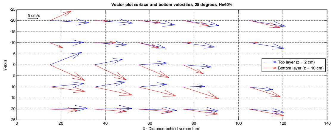
Figure 59 Top view velocity vectors behind the screen
