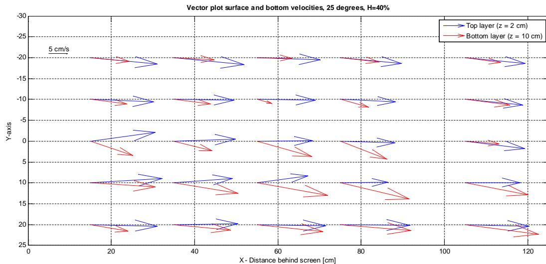
Figure 38 Top view velocity vectors behind the screen
