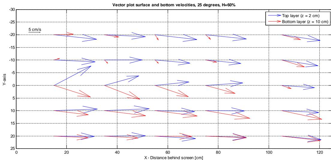
Figure 41 Top view velocity vectors behind the screen
