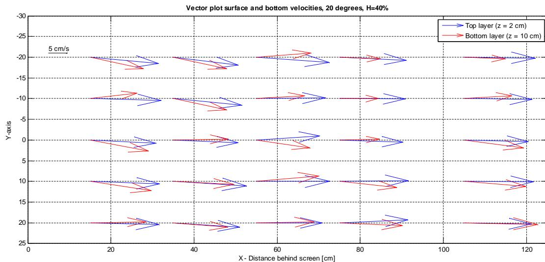
Figure 29 Top view velocity vectors behind the screen
