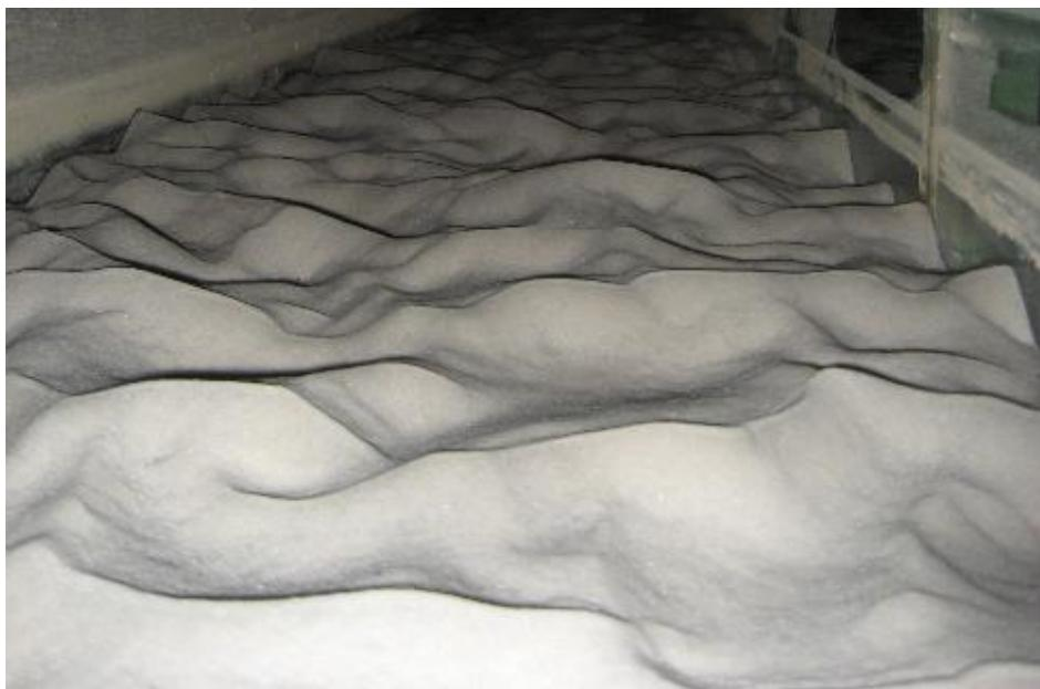
Figure 5 Overview dune structure, looking from downstream in upstream direction
