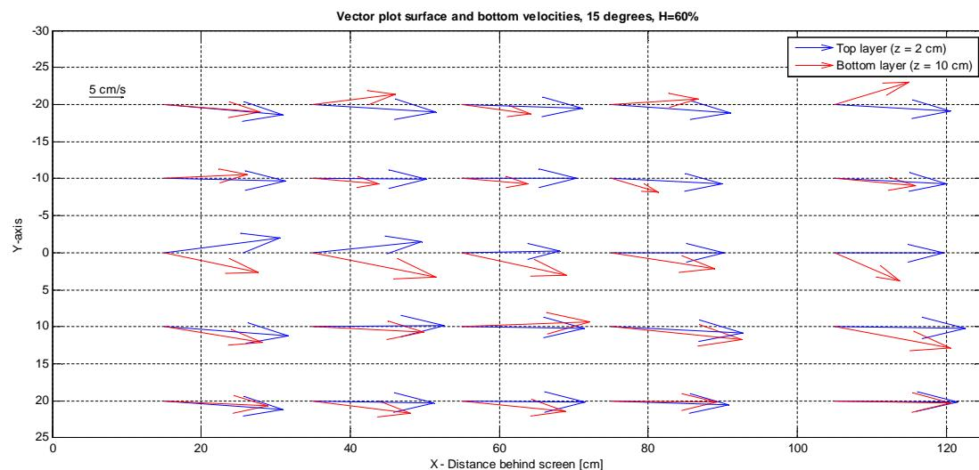
Figure 23 Top view velocity vectors behind the screen
