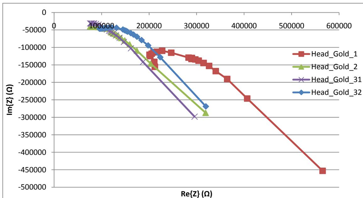
Figure 31. Cole-Cole plot for gold plated electrodes positioned on the head for four successive recording of subject 4 are displayed. The frequencies used in evaluation range from 2 to 500Hz.
