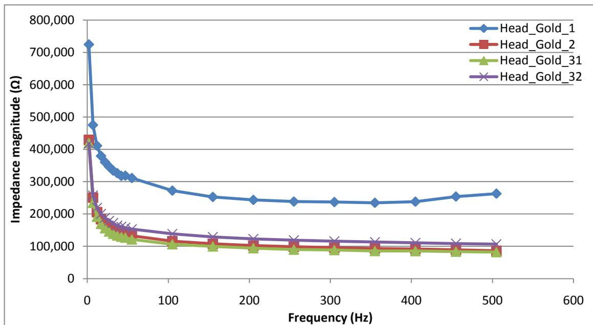
Figure 29. Resistance values for gold plated electrodes positioned on the head of four successive recording of Subject 4 are displayed. The frequencies used in evaluation range from 2 to 500Hz.
