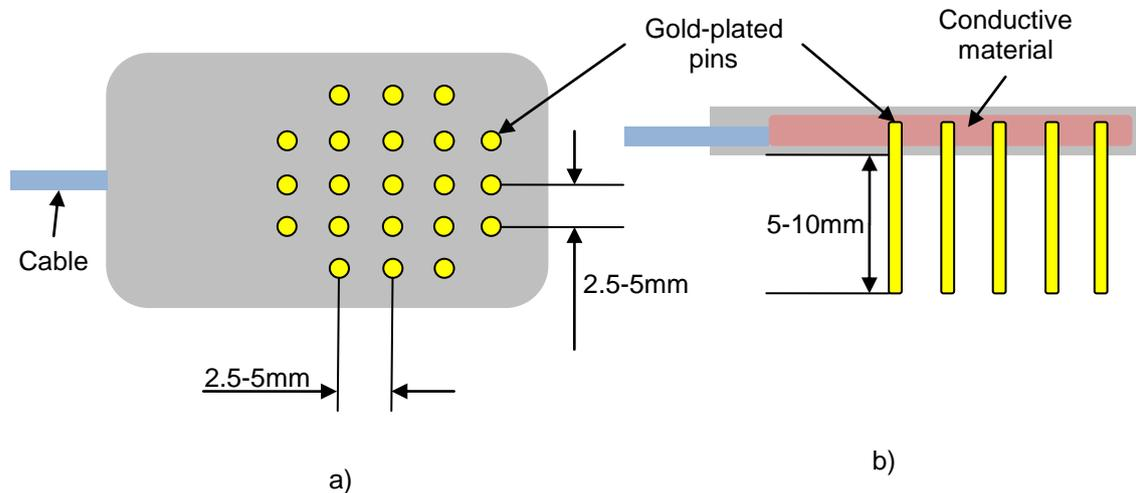
*Figure 3. Schema of the developed gold-plated pin electrodes immersed in the flexible conductive material: a) Bottom view: positioning of the pins in the small support patch; b) Side view: positioning of the pins in the conductive material.*
