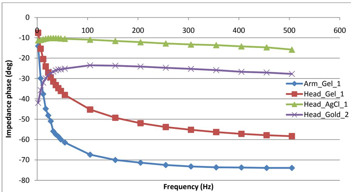
Figure 27. Phase response for Subject 4. Gel electrodes positioned on the forearm and on the head, and Ag/AgCl and gold plated electrodes positioned on the head are displayed. The frequencies used in evaluation range from 2 to 500Hz.
