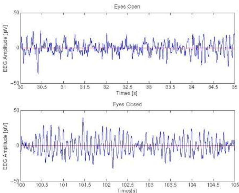
Figure 4. Example of measured EEG signal (high-pass filtered with 1Hz). The top graph shows EEG measured during eyes open and the bottom graph shows the EEG during eyes closed. Alpha activity is clearly visible on the bottom graph.
