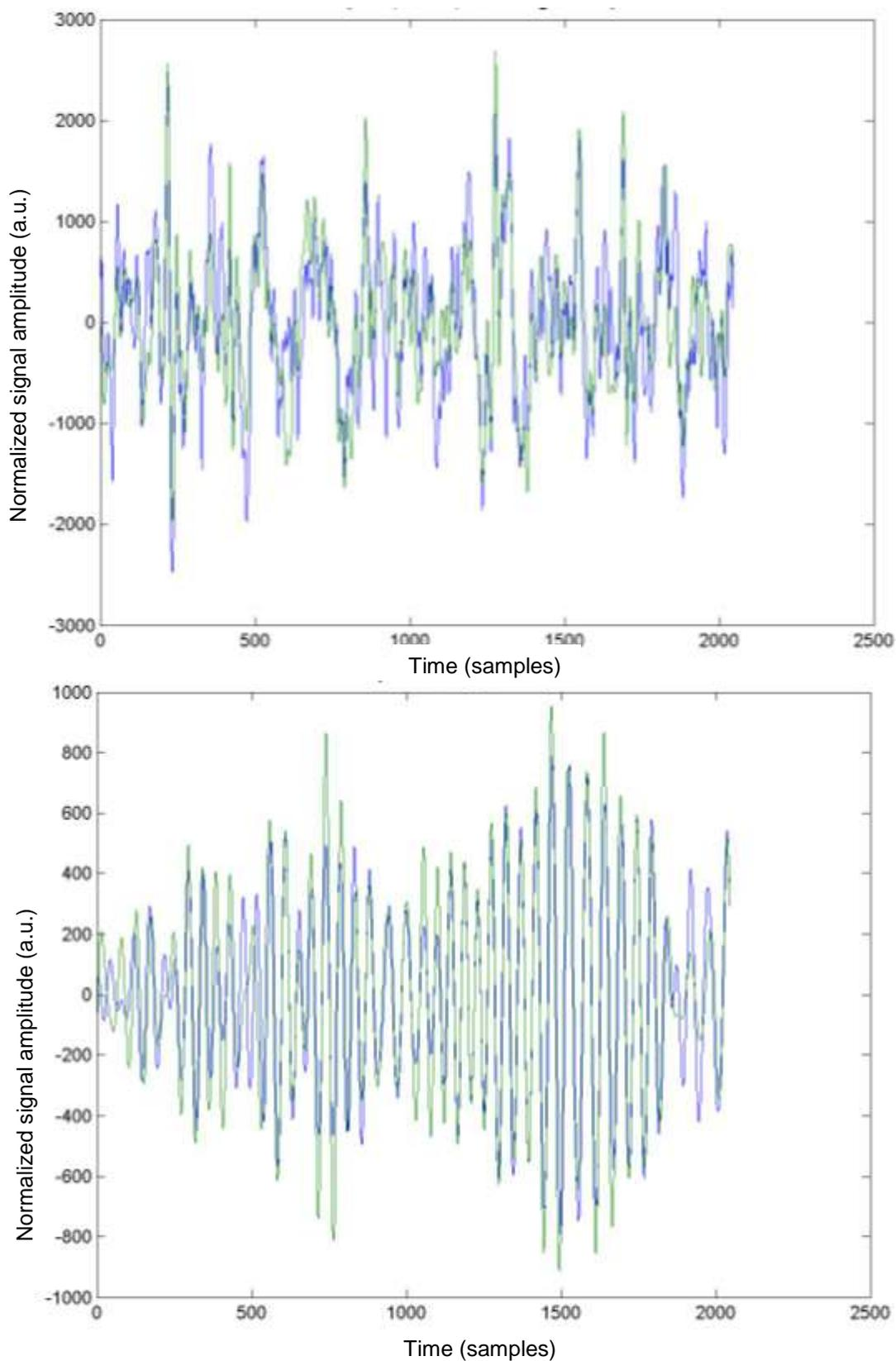
Figure 8. Comparison of the dry (blue line) and wet (green line) electrodes EEG signals, band-pass filtered in the 2-35Hz (top figure) and 8-12Hz (bottom figure). The sampling rate is 512 samples per second. Figures depict 4s recording.
