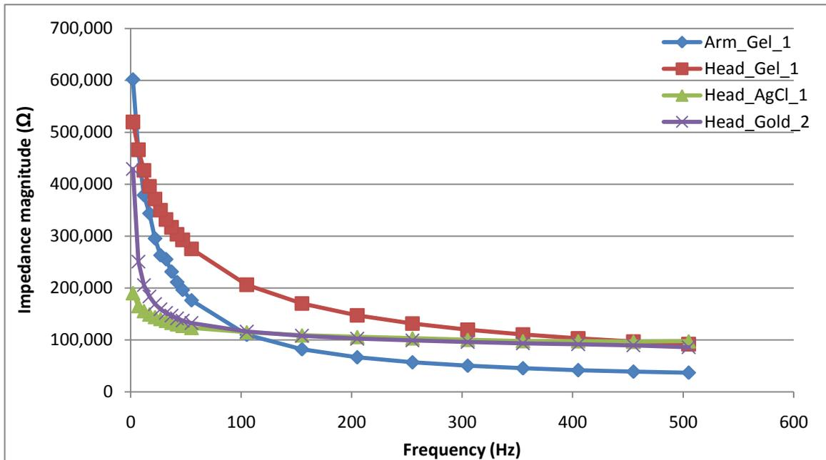
Figure 26. Impedance magnitude values for Subject 4. Gel electrodes positioned on the forearm and on the head, and Ag/AgCl and gold plated electrodes positioned on the head are displayed. The frequencies used in evaluation range from 2 to 500Hz.
