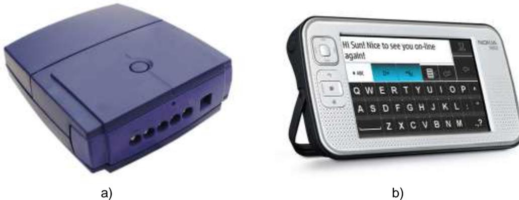
Figure 5. Illustration of the measurement setup: a) TMSi Mobi system used for EEG signal acquisition; b) Nokia N800 used for displaying the signal and signal analysis.
