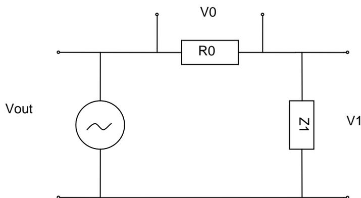
Figure 24. Skin impedance measurement setup.
