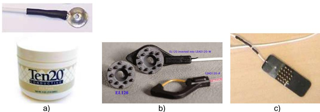
Figure 25. Different electrodes used in the evaluation: a) AgCl electrodes used with gel (gel electrodes); b) dry Ag/AgCl electrodes with pin structure; c) dry gold-plated electrodes with pin structure.
