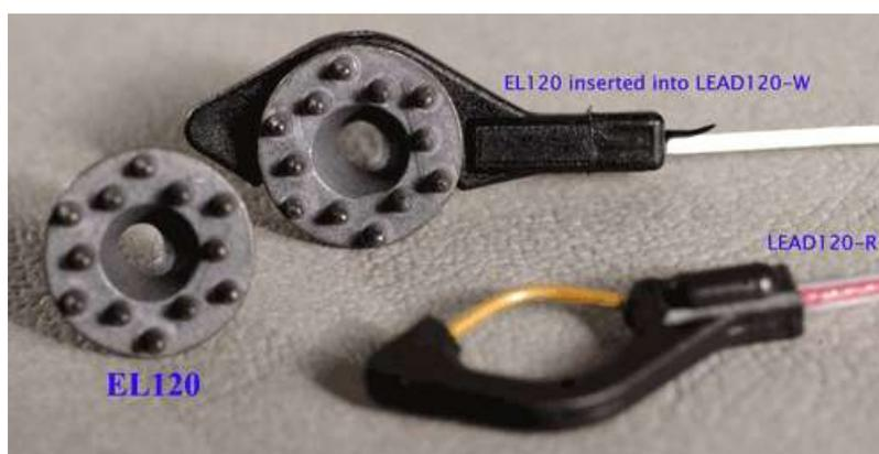
Figure 2. Commercially available sintered Ag/AgCl electrodes with pin structure.
