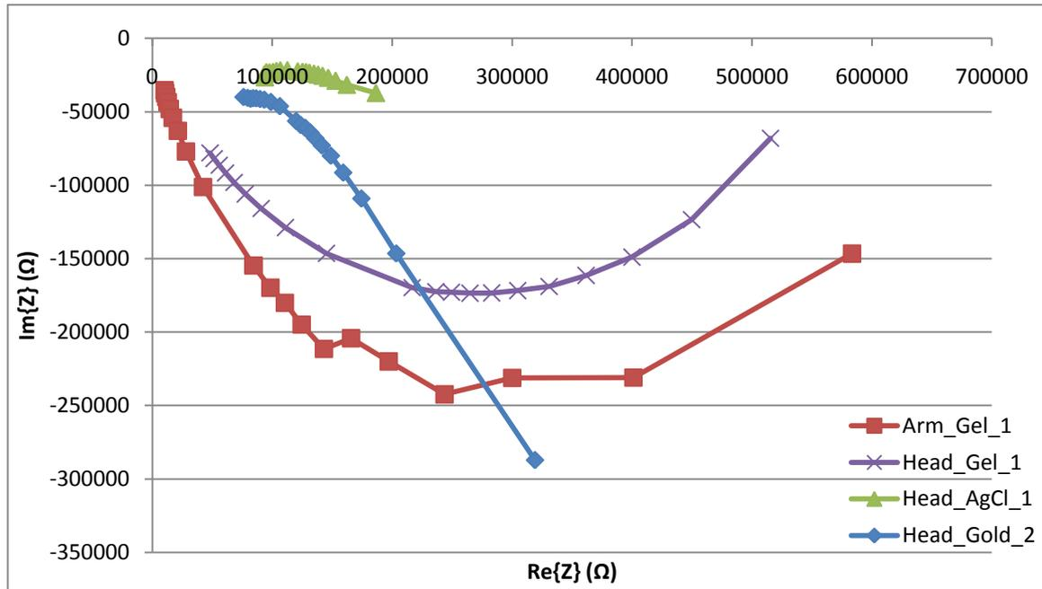
Figure 28. Cole-Cole plot for Subject 4. Gel electrodes positioned on the forearm and on the head, and Ag/AgCl and gold plated electrodes positioned on the head are displayed. The frequencies used in evaluation range from 2 to 500Hz.
