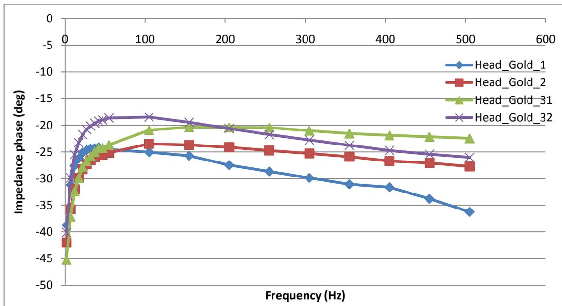
Figure 30. Phase response for gold plated electrodes positioned on the head for four successive recording of Subject 4 are displayed. The frequencies used in evaluation range from 2 to 500Hz.
