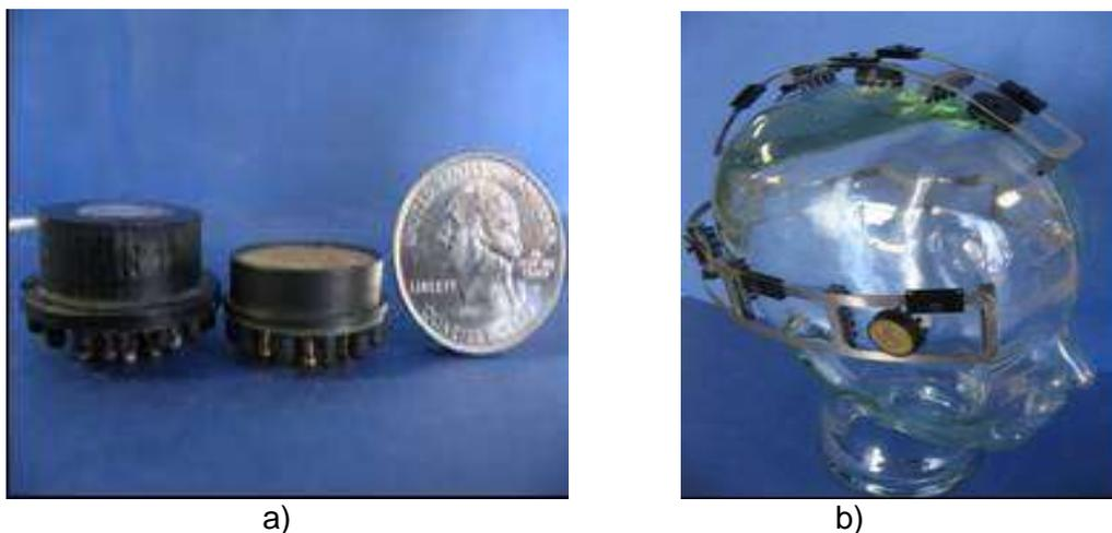
Figure 1. Quasar EEG measurement technology: a) quasar hybrid sensors; b) harness structure that holds the electrodes.
