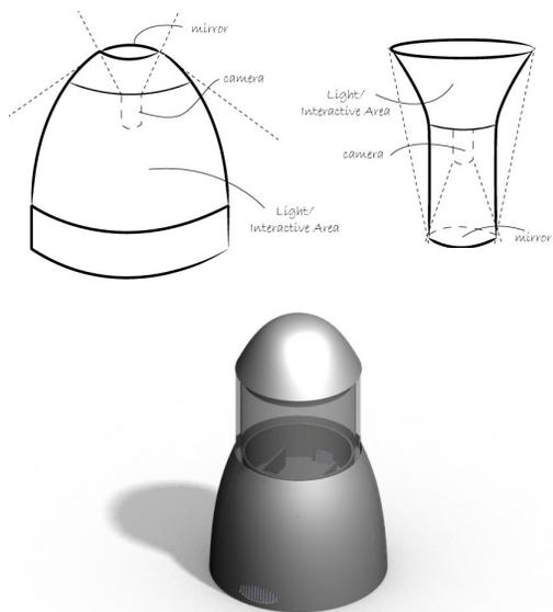
**figure 1.** The SoPresent prototype equipped with a microphone, camera and a mirror to provide a 360 view for context determination.
