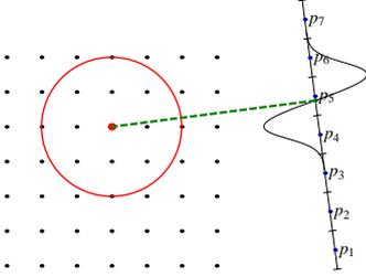
FIG. 2: Illustration of forward projection using blobs. A sample blob (thick red dot in the image grid) has a support as indicated by the red circle. The contribution of this blob to the differential projection is obtained by forward projection of the blob center to the detector (dashed green line) in order to determine the relative position of the differential footprint to the detector and to sample the pre-tabulated differential footprint at the detector pixel centers  $p_i$ .
