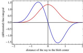
FIG. 1: Footprint of a Kaiser-Bessel blob and its derivative for  $a = 2$ ,  $m = 2$ , and  $\alpha = 10.826$ .
