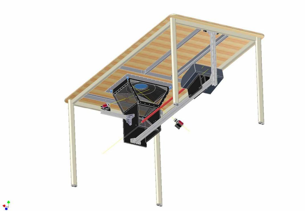
*Figure 29: Bottom view of the set-up as designed in Autodesk Inventor. Notice the extra beams underneath the table to strengthen it. In this picture is also visible how the video projector is connected to the table and the tank.*
