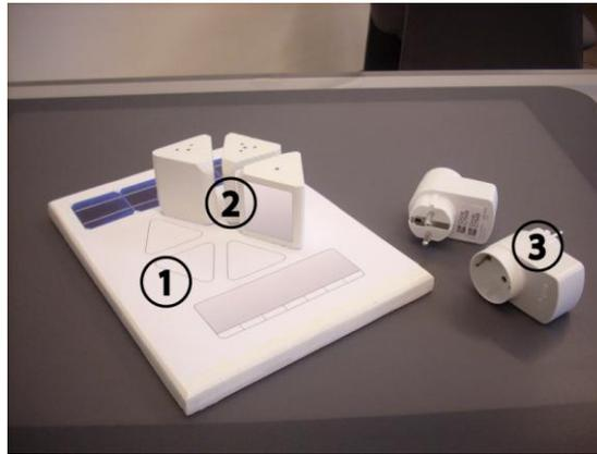
**Figure 1.** The basic elements of the Flo concept: 1) Docking station, 2) Personal "cubes", 3) Plugs with sensors.
