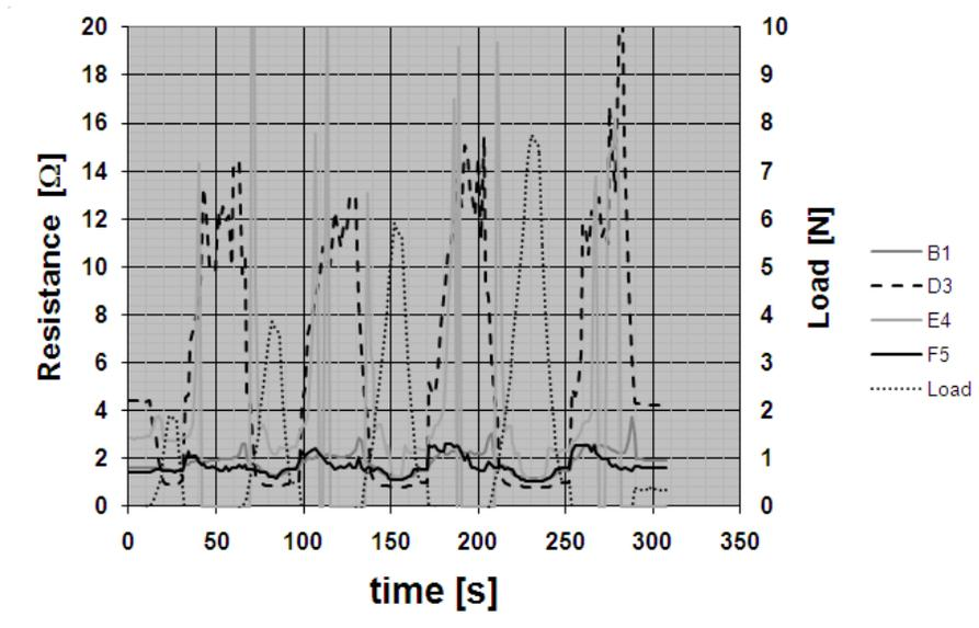
Fig. 6. Resistance of eight contacts in *fabric B* as a function of time, tested in the warp direction
