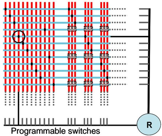
Fig. 4. Schematic representation of the programmable resistance measuring method
