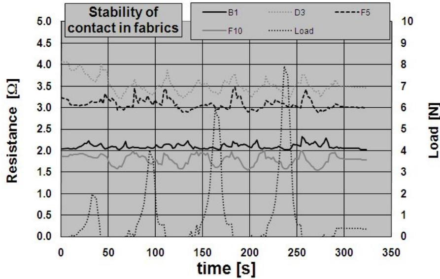
Fig. 9. Resistance of ten contacts in *fabric J* as a function of time, tested in the warp direction
