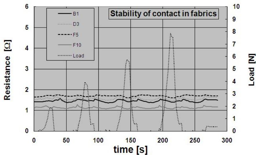
Fig. 8. Resistance of ten contacts in *fabric H* as a function of time, tested in the warp direction
