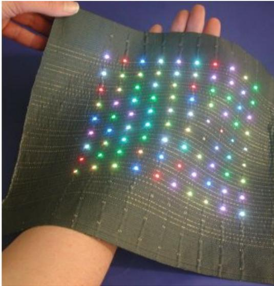
Fig. 12. Light-emitting fabric: conductive yarns are interwoven with polyester yarns and LEDs are attached at the crossovers
