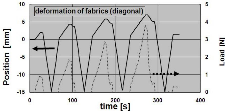
Fig. 5. Measured displacement during the four subsequent loading cycles in a (diagonally) tested fabric.
