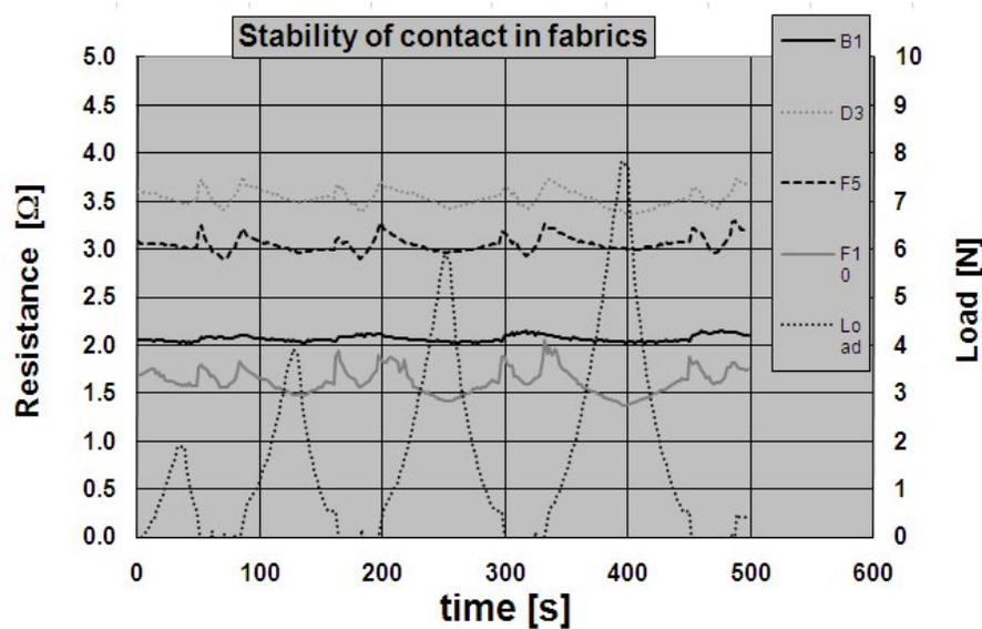
Fig. 10. Resistance of ten contacts in *fabrics H (left) and J(right)* as a function of time, tested in the weft direction
