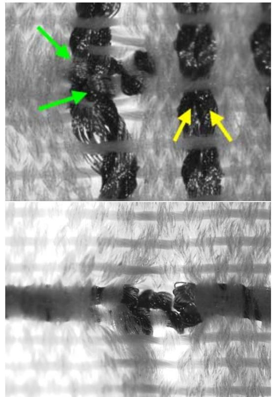
Fig. 11. Via contact in fabric H, observed from (a) backside, and (b) front side of fabric
