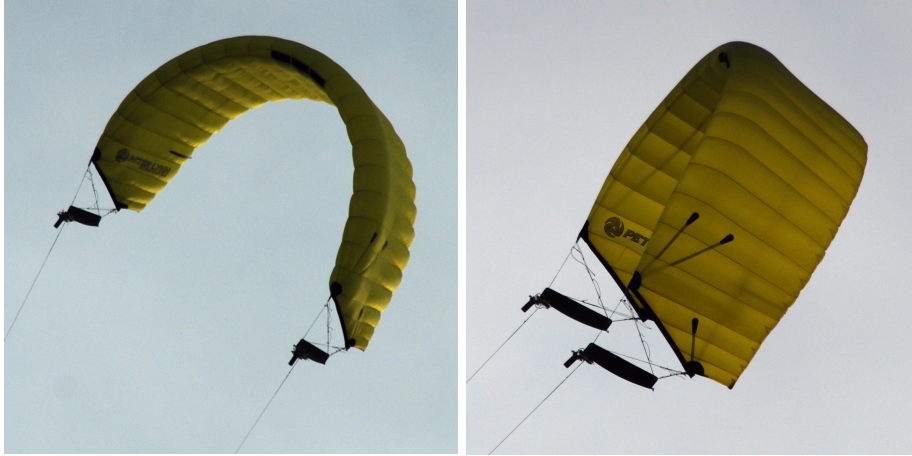
Figure 1: Two-line kite with rack-and-pinion system to move tip attachments of lines [13]
