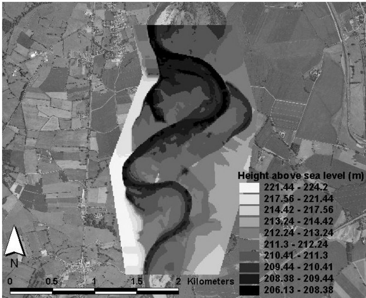
**Figure 6.3:** Bed topography and model domain of the study area. Flow is from south to north. Height relative to sea level (m).
