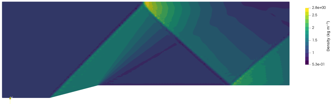
Figure 3.14: Run 2: wedge case with the Fejér filter for run 2. Detail of the attached shock on the wedge.
