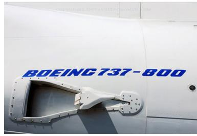
Figure 13.36: Example of a NACA Duct from the Boeing 737-800<sup>20</sup>
