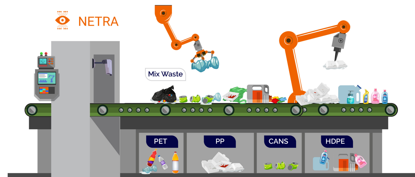
Figure 24 AI driven sorting machine
