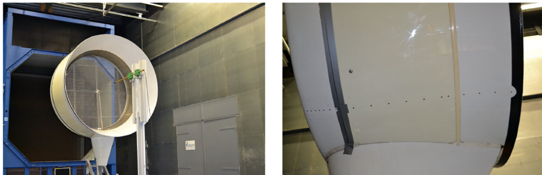
FIGURE 2 Pictures showing the experimental set-up with hot-wire anemometer placed on the traversing system (left) and pressure taps along the duct surface (right) [Colour figure can be viewed at wileyonlinelibrary.com ]
