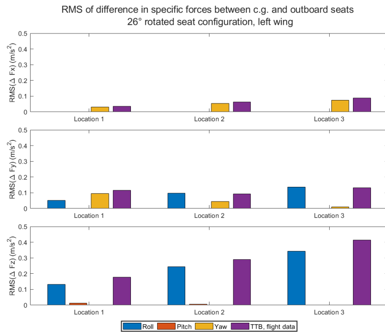
Figure 4.29: RMS Specific forces differences for the left wing, 26° rotated seat configuration
