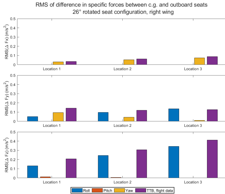
Figure 4.30: RMS Specific forces differences for the right wing, 26° rotated seat configuration
