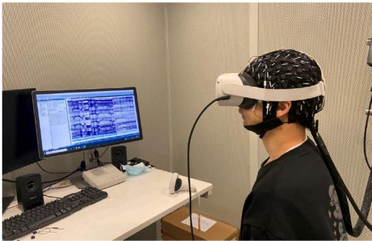
Fig. 4. The EEG collection environment. The EEG data was collected in a soundproof room. Subjects wore a cap fitted with 128 electrodes and put on a VR headset at the same time.
