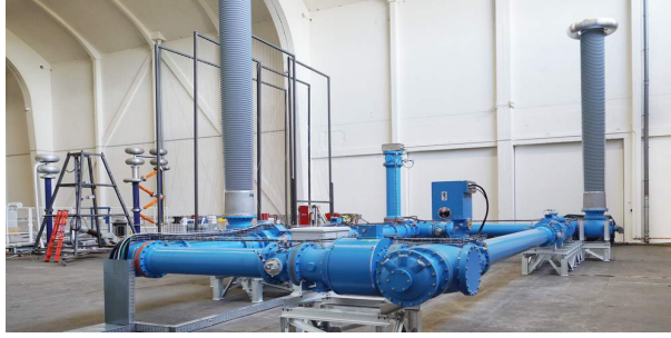
Figure 3: PROMOTioN Project ABB's 320 kV HVDC gas insulated switchgear (GIS) test equipment in the KEMA High Voltage DC Laboratory in Kleefse Waard, Arnhem, Netherlands. [6].
