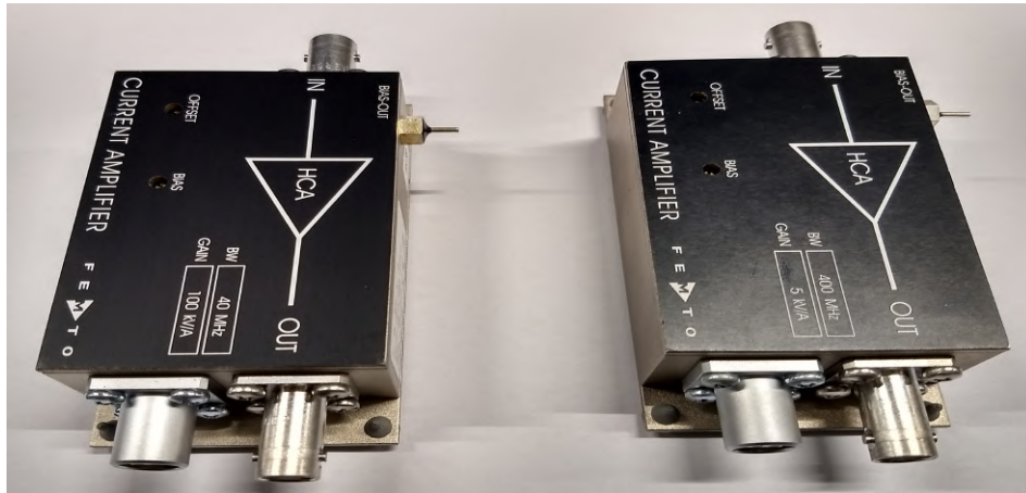
Figure 19: 40M-100K (left) and 400M-5K (right) Femto Current Amplifiers
