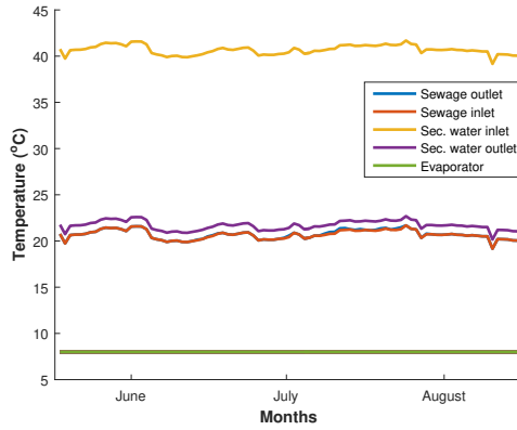
Figure 60: WWSHP Summer model : Temperatures of different streams
