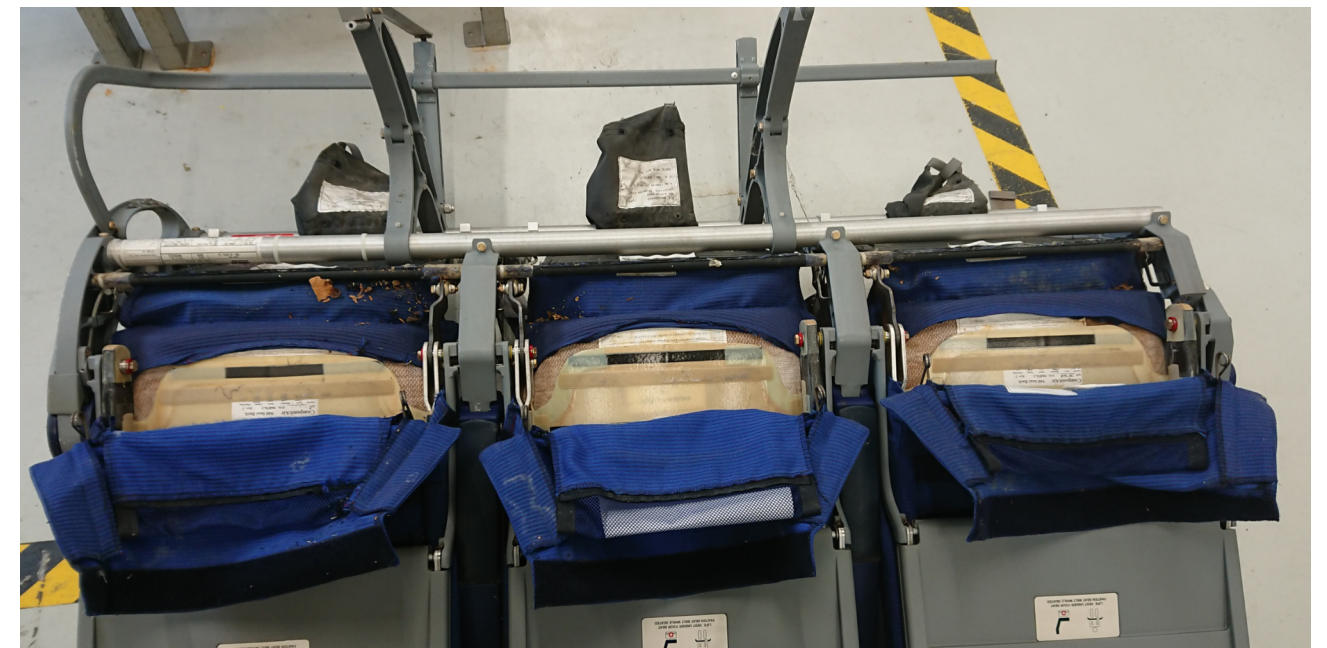
Fig. 27. Non-structural part assembly 8 Almost no tools were needed to disassemble the non-structural parts. The seat cushions and upholstery were all attached with Velcro, making disassembly very simple. This is probably for ease of maintenance as there was a label on the upholstery to indicate when the fabric was last cleaned.
