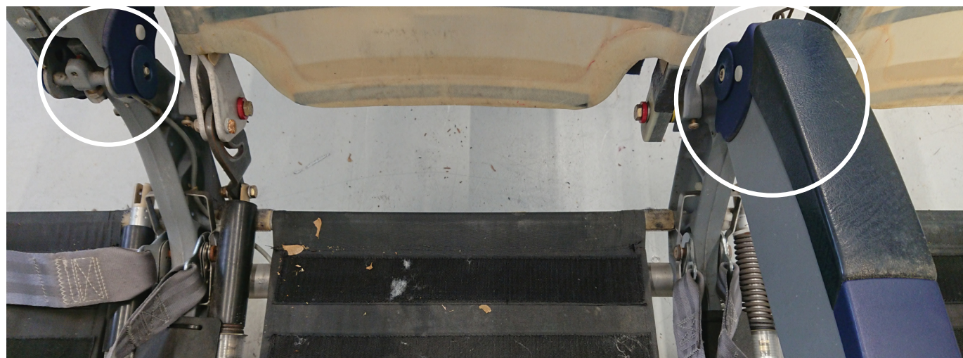
Fig. 26. Structural part assembly 7 The armrests are bolted at the top of the spreaders and house the button that controls the hydraulic spring of the recline mechanism. Both English and metric bolts were used in the seat construction. Many bolts also had varying sizes. This required several different tools to disassemble the seat. Apart from a few oxidized bolts, however, everything was relatively easy to disassemble without having to destroy any part of the seat.
