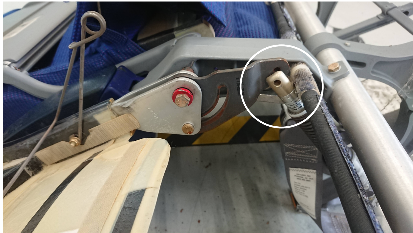
Fig. 25. Structural part assembly 6 The above mechanism limits the recline angle and is attached to the hydraulic spring on the right.
