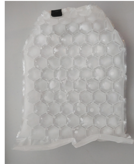
Figure 1: Crumpled band due to filling the pack.
