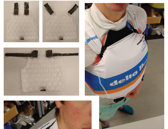
Figure 2: The shoulder bands of the flotation aid are too flexible to carry an ice pack.
