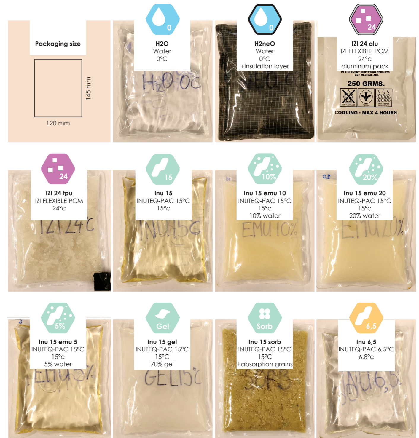
Figure 2: Overview of the PCM samples that were tested on the Hotplate.
