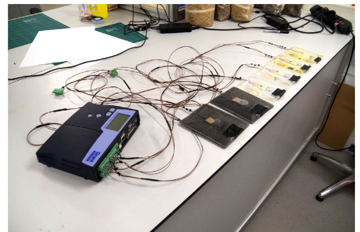
Figure 4: Six samples with a thermocouple in the center and at the surface.
