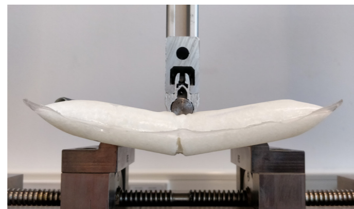
Figure 3: Sample at the end of a three point flexural test on the tensile tester.
