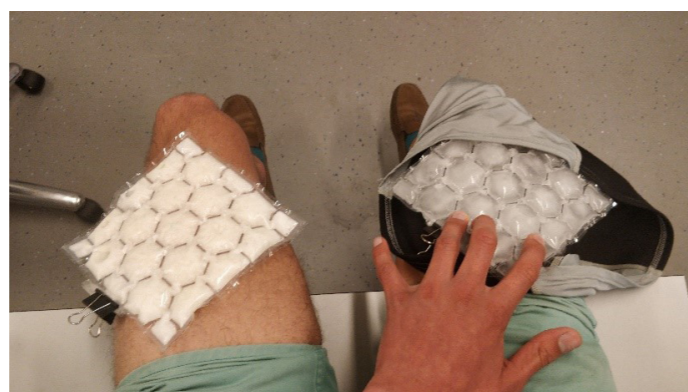
Figure 1: Ice with a Neoprene shirt feels about equally as cold as PCM Inu 15°C.
