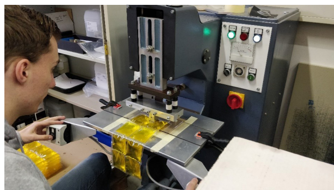
Figure 1: 8-cell PCM packages and ultrasonic welding machine used to attach Velcro.
