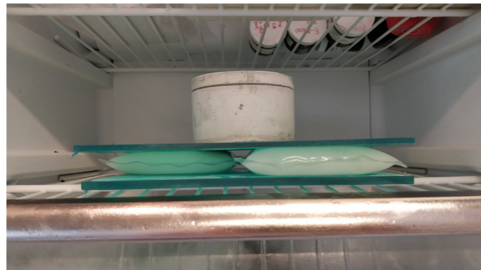
Figure 1: Cooling of samples while compressed between two Perspex plates
