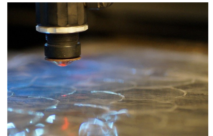
Figure 2: Laser cutter used for sealing and a close up photograph of the laser head above sealed foil.
