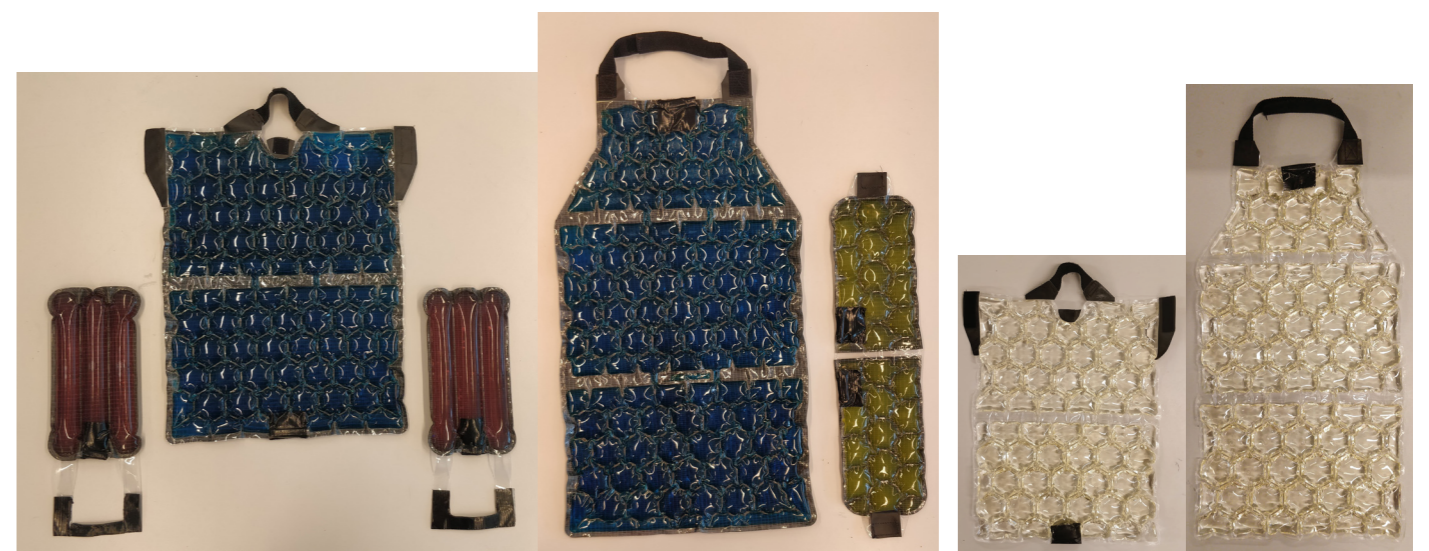
79 Figure 4: Prototype 6, the version with H2neO (blue) is shown on the left, together with the side (red) and neck (yellow) packs. The inu 15 version (transparent) is shown on the right.
