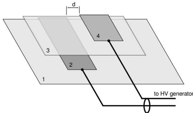
Figure 1. Actuator layout. 1 — base insulation layer, 2 — covered electrode, 3 — inter-electrode insulation layer, 4 — exposed electrode,  $d$  — gap width.
