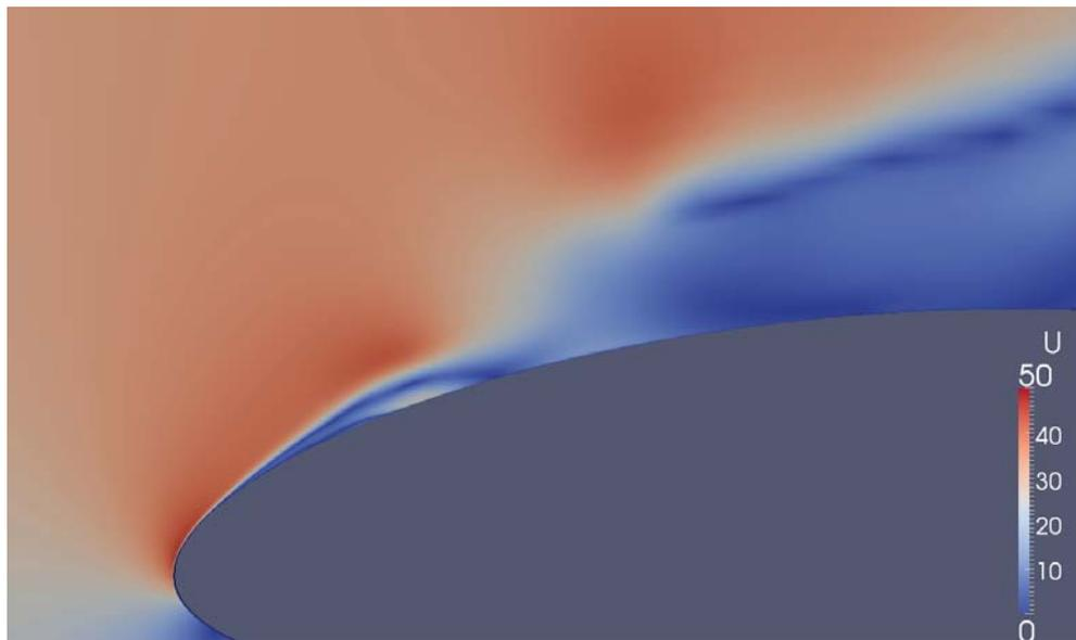
Figure 5. Simulation of the laminar separation with actuation: velocity field after the discharge. Magnitude of the velocity is shown by color.
