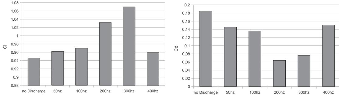
Figure 3. Lift and drag coefficient at different discharge frequencies.  $V = 20$  m/s,  $\alpha = 15^\circ$
