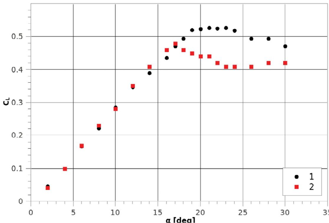
Figure 2. Lift curves of NACA0015 wing at  $V = 30$  m/s. Actuator turned on (1) and off (2). Note that the lift coefficient as well as the angle of attack have not been corrected for open jet wall effects.
