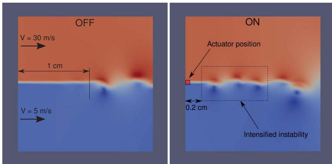
Figure 6. Velocity field without and with actuation in shear layer simulation. Thickness of shear layer at the inlet is 0.5 mm.
