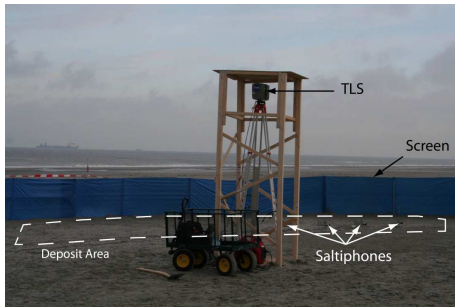
(a) Experiment setup: sand particles transported towards the plastic screen and the wooden house protecting the terrestrial laser scanner Faro Photon 120.
