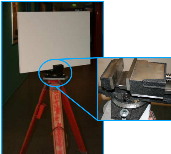
Figure 5.6: Reference plate measurement set-up. A white coated plywood board is mounted on a tripod via a screw clamp mechanism provided with a 2^\circ precision goniometer.
